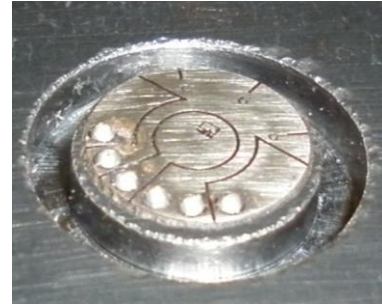
Figure 15: On the left, the results obtained with the differential method at the various measurement points on the forging. On the right, a typical annular groove made by the instrument.
