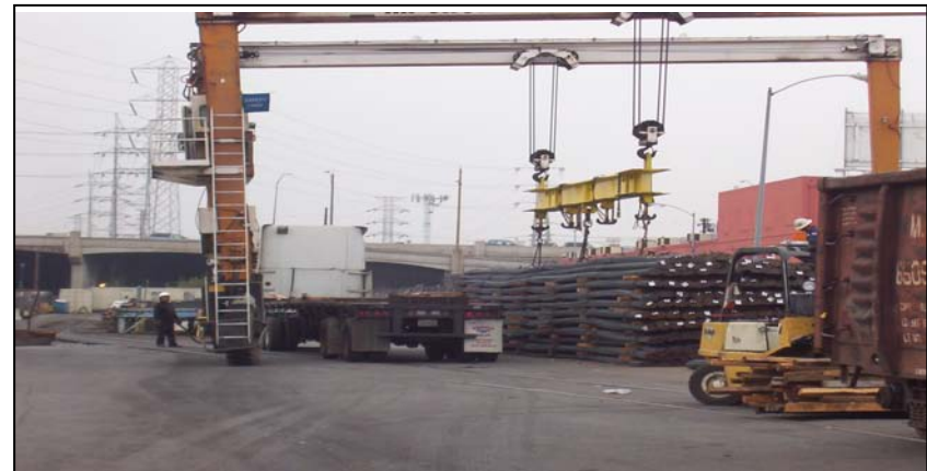
Transload from yard storage to truck (Product arrived by rail several days earlier)
