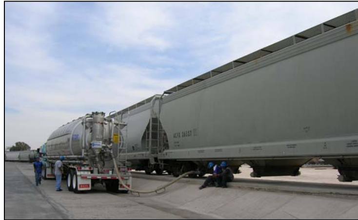
Bulk transload from rail car to truck
