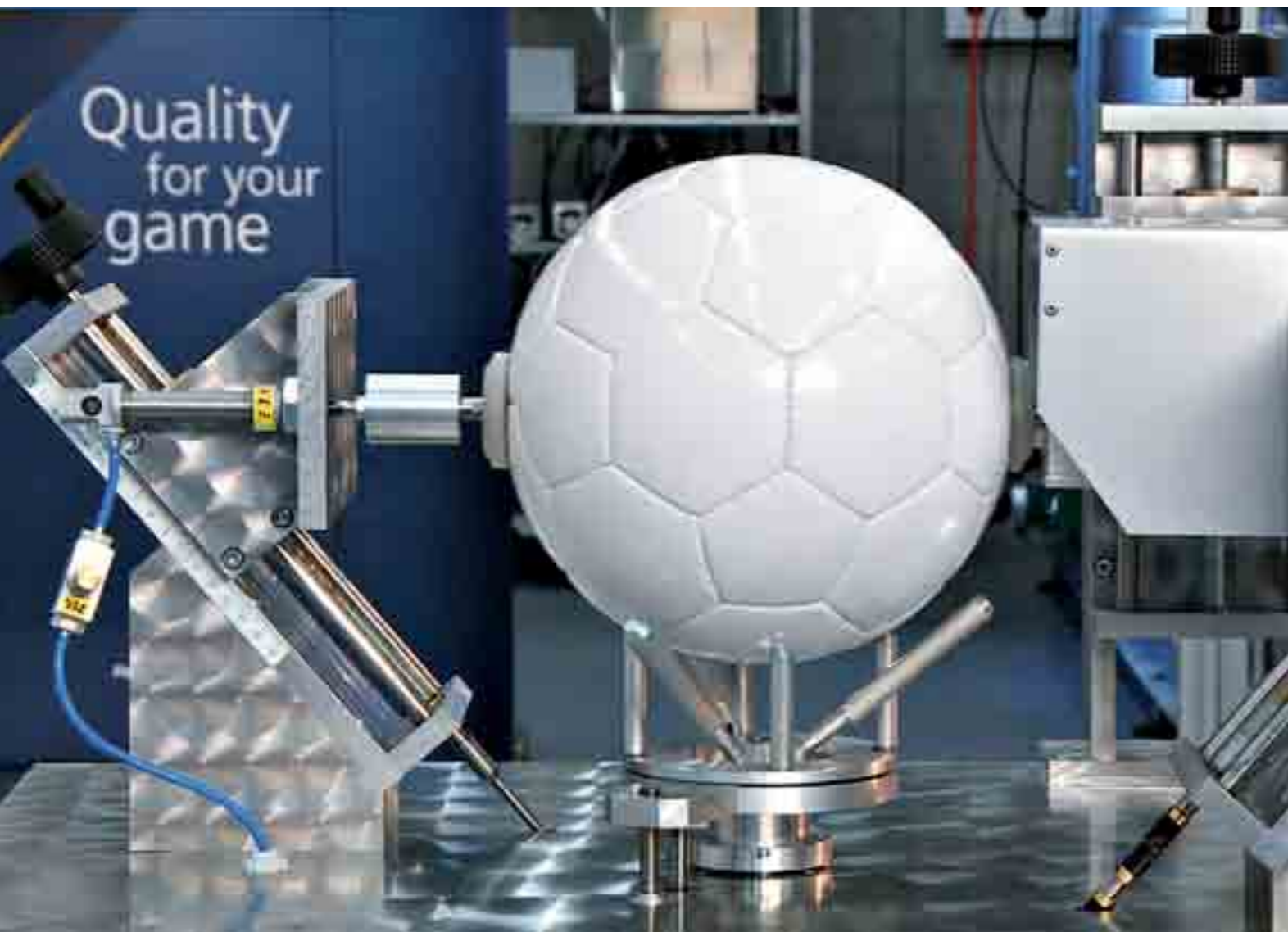
The sphericity and quality of the ball are no longer measured by hand, but fully automatically.
