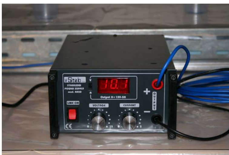
Figure 3.2 – DC generator Stab AR50 used in the experimental investigation (providing a stabilized DC up to 15 V and up to 5 A).
