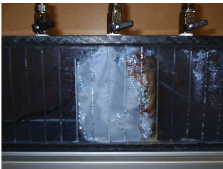
Figure 4.74 – Kaolin sample being treated with Setup 2: at the anode (on the right side of the sample), the soil was compacted and changed to a yellow-orange color because of the formation of iron hydroxides from the soil natural iron content and from the electrode corrosion.
