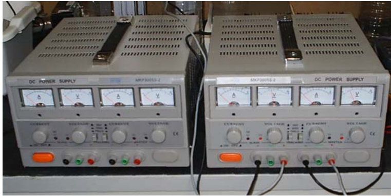
Figure 3.3 – Two DC generators Mitek MICP 3005S-2 used in the experimental investigation (each one providing a stabilized DC up to 60 V and up to 5 A).
