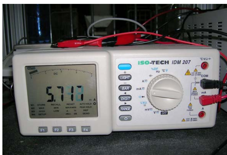
Figure 3.16 – Digital multimeter ISO-Tech IDM 207 for continuous current monitoring.
