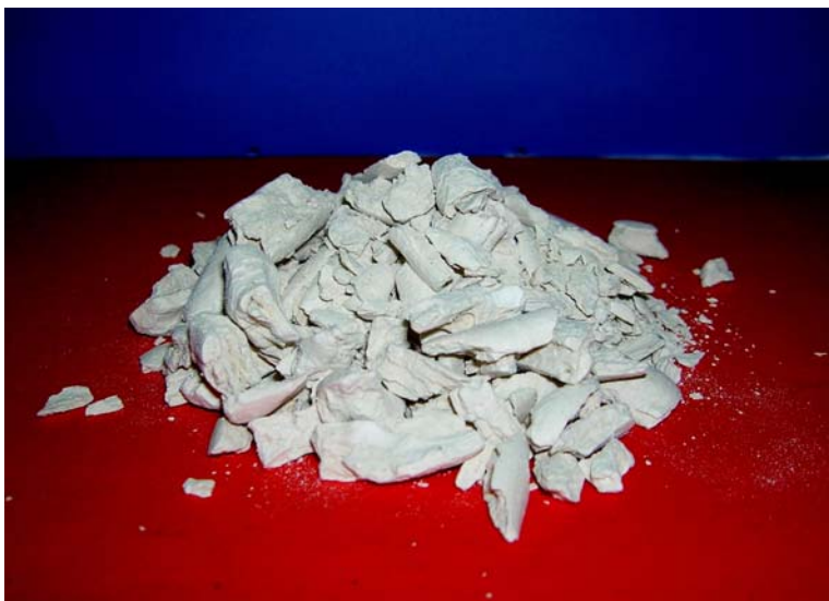
Figure 4.2 – Sample of bentonite used for the experimental investigation.
