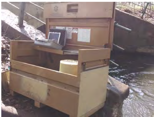
Figure 26-2. Top: Xerxes monitoring station location at Minnehaha Creek. The staff gauge is a vertical white line in the middle right. Left: Knaack installation with sampler and datalogger. Right: Close up of intake strainer and level probe anchored to the northwest bridge abutment.
