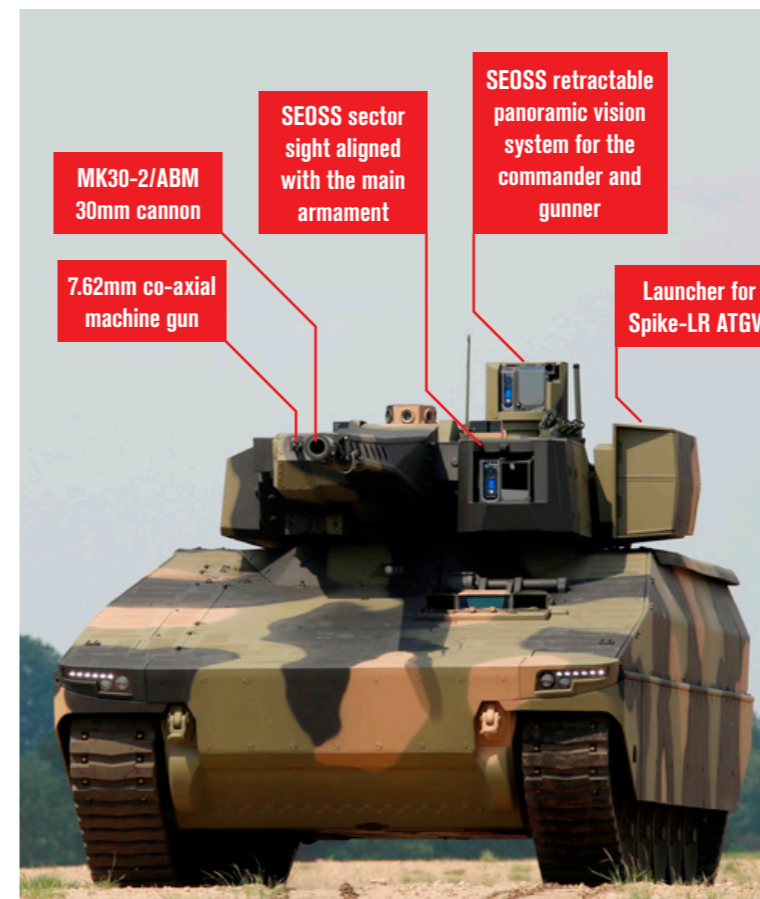
LEFT: Advanced sighting systems for the commander and gunner, the option of a 30mm or 35mm main armament and a fully-integrated turret-mounted ATGW render the Lynx IFV a highly lethal platform.
