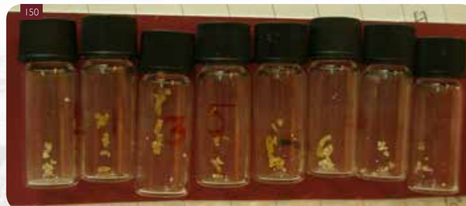
The vials have to be stored cold in the field and frozen (-20°C) in the lab before they can be sent for analysis
