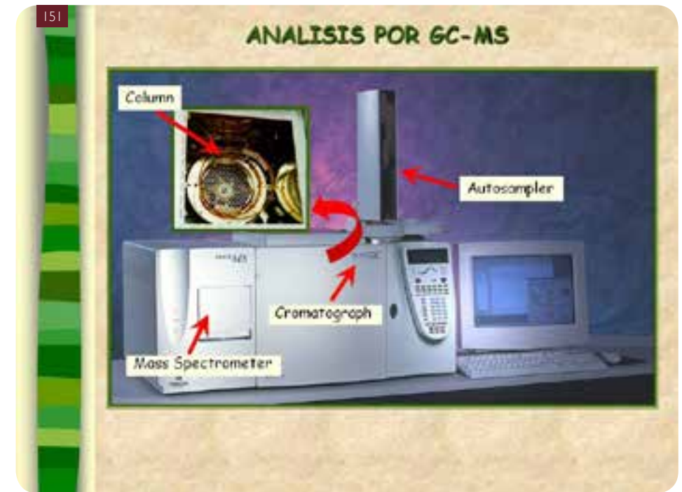
ThermoQuest Trace 2000 gas chromatograph from the Physiology laboratory at the National Museum of Natural Sciences (Spanish National Research Council, CSIC) in Madrid (Spain) that was used to analyze the chemical compounds of the Dhub secretions in Qatar (Martin et al. 2011)
