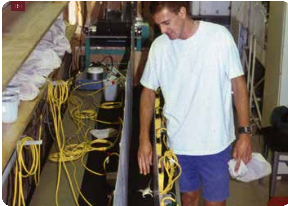
181 Photocell-lined racetrack connected to a computer used to measure maximal running speeds of lizards. Lizards are chased by hand which simulates a predator
