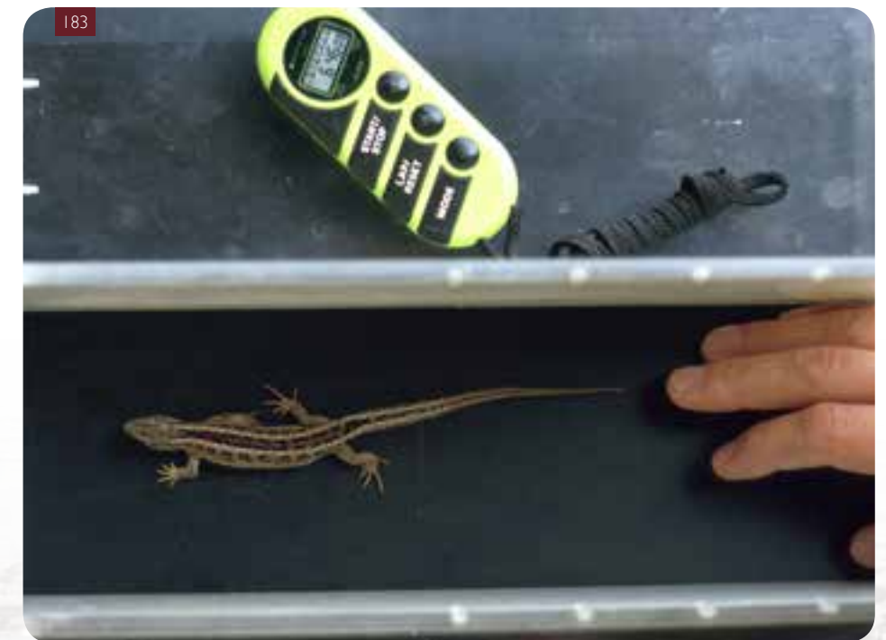
183 Motorized treadmill used to measure endurance in lizards. The standard speed of the treadmill is 1.0 km/h. The length of time the lizard can run at this speed is taken as the measure of endurance. The lizards are chased to keep them moving
