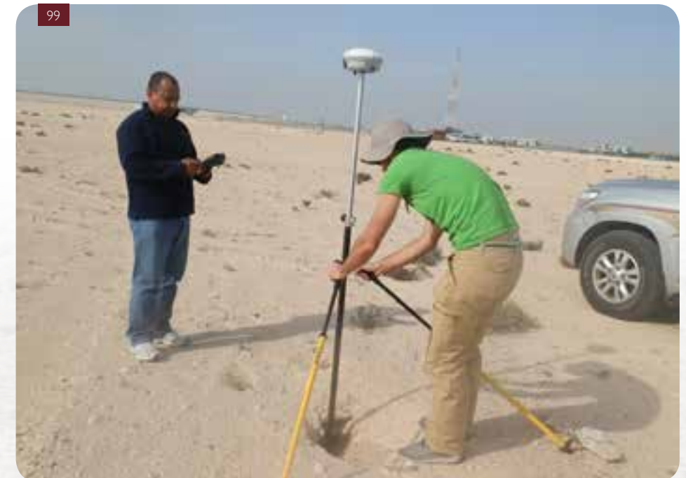
High accuracy GPS (Trimble Real Time Kinetic RTK8) property of Qatar Foundation used for more detailed geographic positioning
