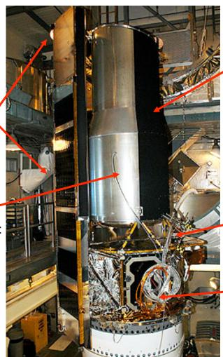
High emissivity surface for radiating heat: T~30 K
