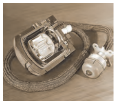
Bottom. IOAV and IOAV-2 spectrophotometers, which measured the content of water vapour in the atmosphere of Venus
