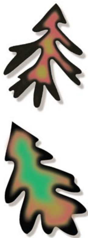
> Models of a sun leaf made of a liquid crystal sheet with a temperature range of 30° C (black) to 35° (blue); the two models have been subjected to the same mild radiant heating from above with negligent airflow at an ambient temperature of 21° C.
