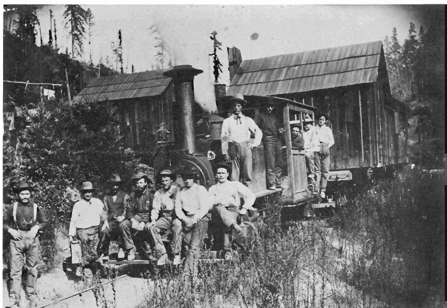
Albion Lumber Company engine Number 4, 0-4-0T, "The Goat", switching the mill at Albion.
