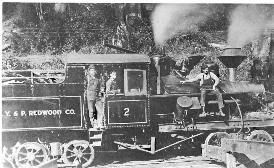
New York & Pennsylvania Redwood Company engine Number 2, a double-truck Heisler, which later became Navarro Lumber Co. engine Number 2.
