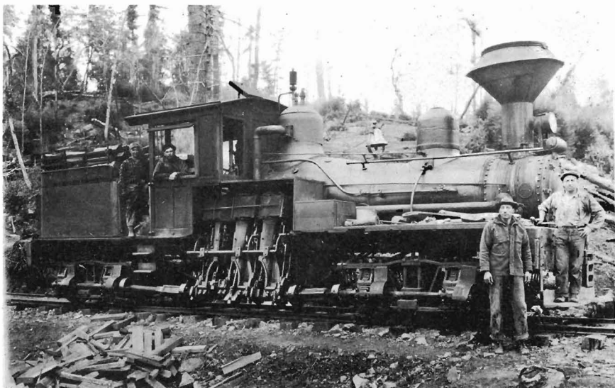
Albion Lumber Company engine Number 1, double-truck Shay, at Perry Gulch with Oscar Newman as engineer. Collection of Oscar Newman
