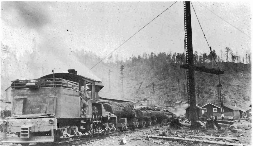
Albion Lumber Company engine Number 1, double-truck Shay, working at Camp A in Perry Gulch with Oscar Newman as the engineer.
