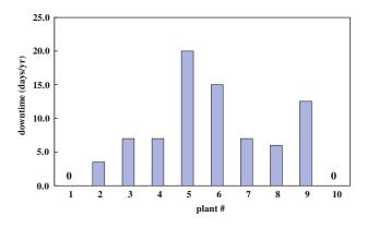
**Fig. 3** Non-scheduled downtime due to corrosion of waste-to-energy (WTE) plants (A1, B1, etc. refer to different waste-to-energy (WTE) facilities responding to the WTERT survey)
