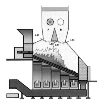
Fig. 8 Schematic diagram of the Seghers Boiler Prism
