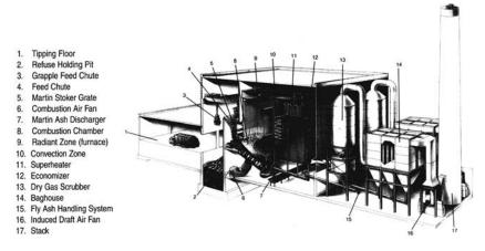
Fig. 1 Schematic of typical waste-to-energy (WTE) facility
