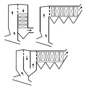
Fig. 7 Schematic diagram of vertical and horizontal boilers
