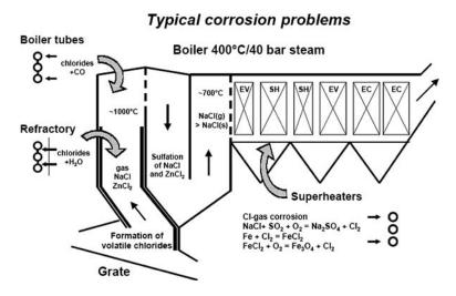
Fig. 2 Corrosion sensitive areas in waste-to-energy (WTE) boilers
