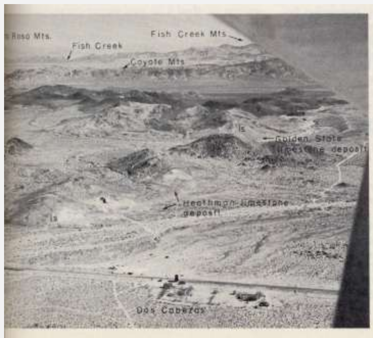
“Photo 46. Aerial view north-northwest, showing Dos Cabezas area and vicinity. Layers of Crystalline limestone (ls) with quartzite and schist are intruded by tonalite (quartz diorite, †) and overlain partly by volcanic flows (Alverson andesite, v), Elsinore fault strikes northwest along base of south side of Coyote Mountain. Parts of Fish Creek gypsum deposits are exposed along crest of ridge just to right of Fish Creek.” (pp. 173)
