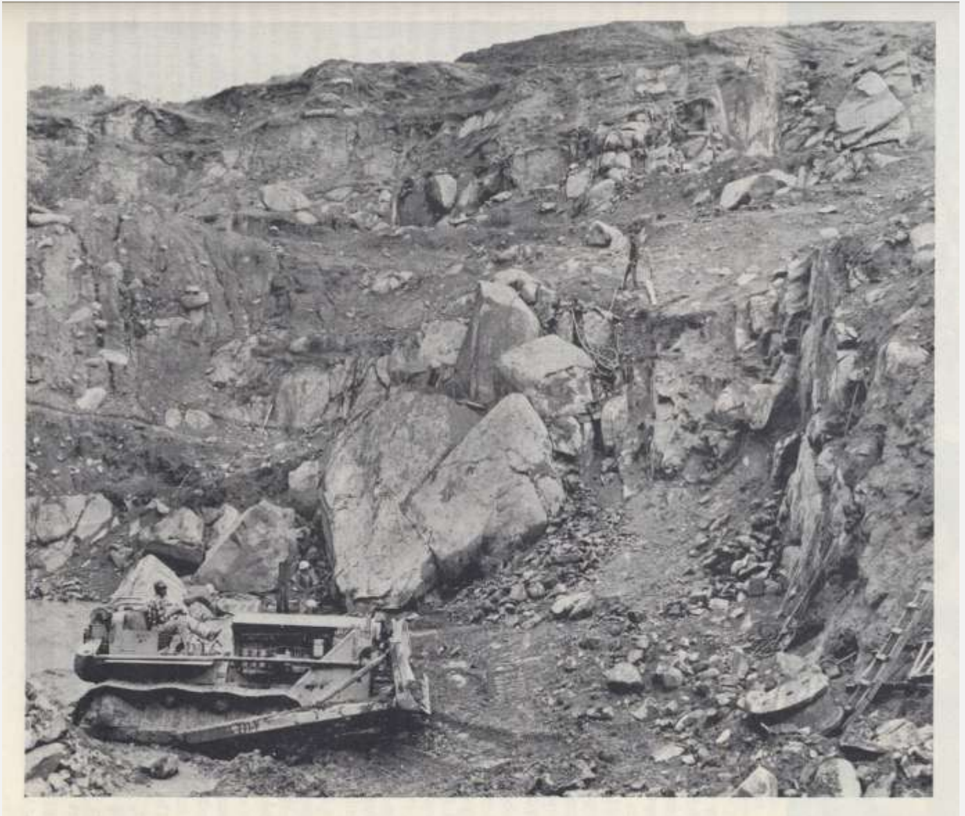
“Photo 82. Escondido-Quarries, Inc., Harmony Grove. Residual boulders of gabbro (black granite) are blasted, then worked downward toward quarry floor which is west (left) of area photographed. Boulders are as large as 25 feet in diameter. Photo by Mary Hill.” (pp. 259)
