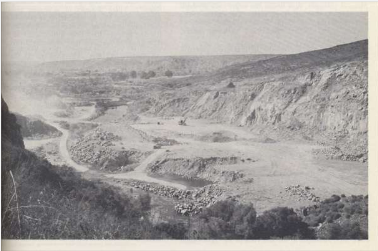
“Photo 75. Canyon Rock Company operation of V. R. Dennis at Mission Gorge; view southwest. Company produces sand from bed of San Diego River (left background) and crushed stone from massive metavolcanic rocks shown in quarry walls. Mission Valley is at left in distant background.”
