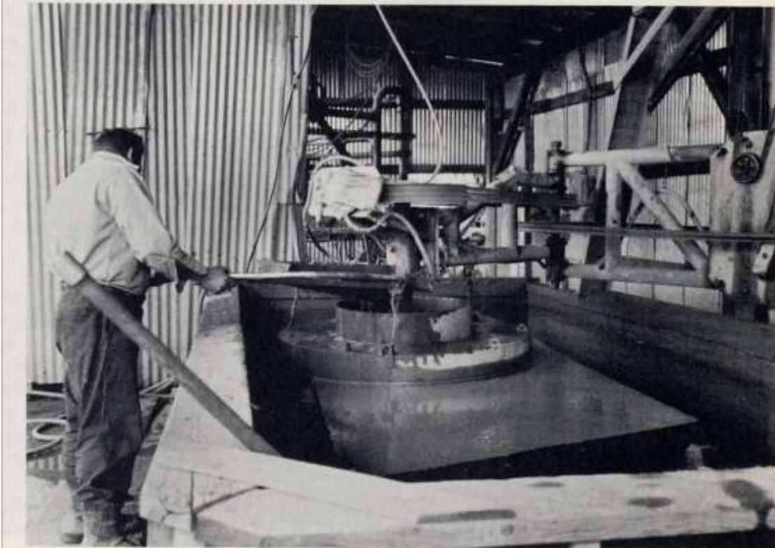
Photo 81 (below). Polishing slab of black granite at Escondido Quarries, Inc. operation of Pacific Cut Stone Co. Photo by Mary Hill.
