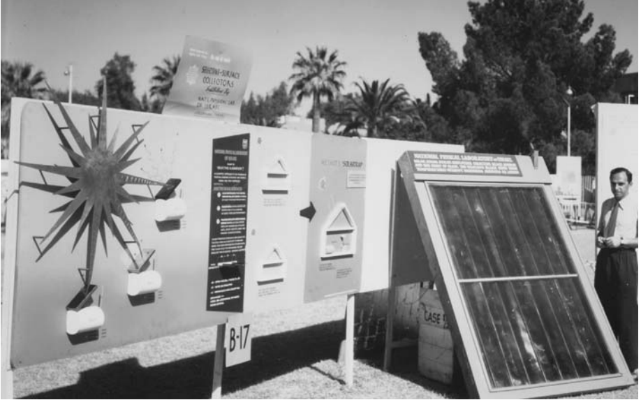
Fig. 6: Harry Tabor with a flat-plate selective-surface steam generator at the “Sun at Work” exhibition at Phoenix in 1955
