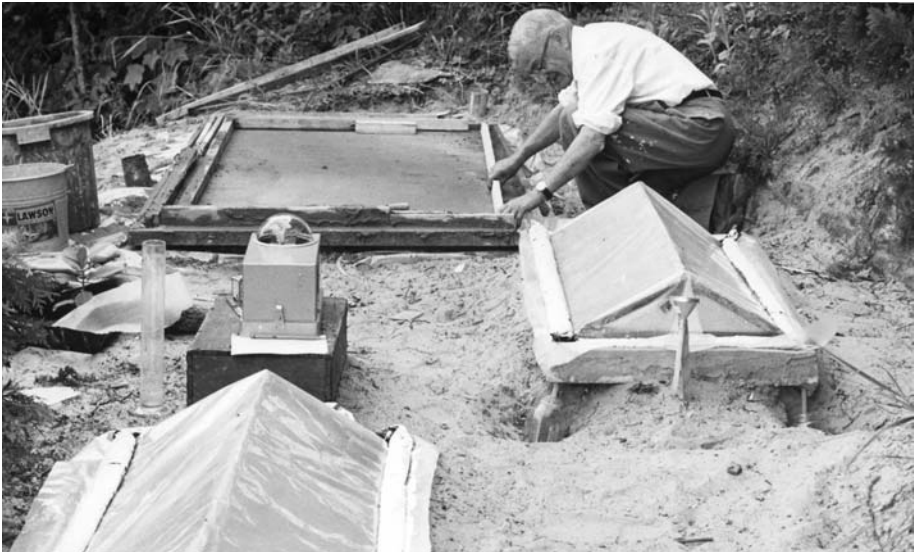
Fig. 21: Farrington Daniels experimenting with solar stills at his summer home in Wisconsin
