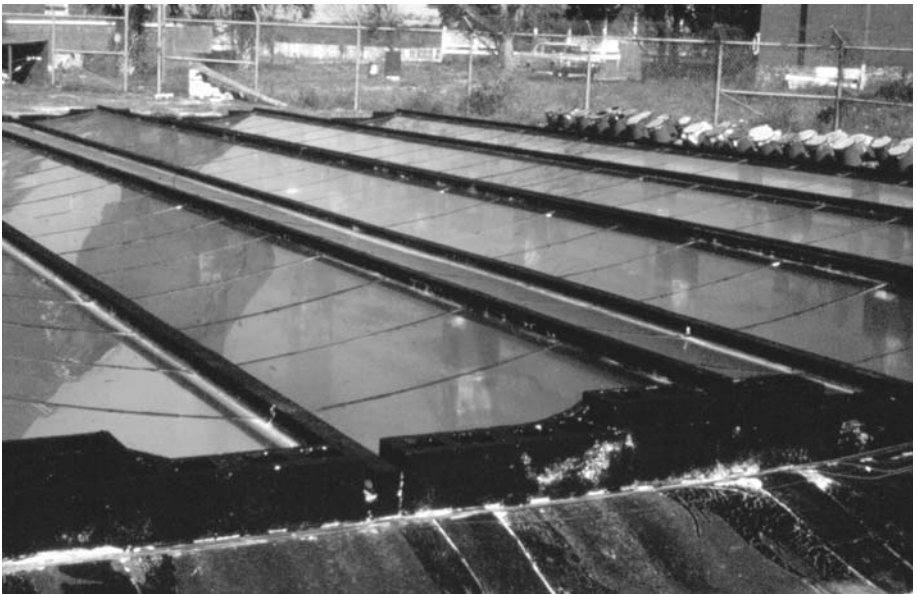
Fig. 14: Deer-layer solar still designed by George Löf at Daytona Beach, Florida. This and other experiments were noted in AFASE publications
