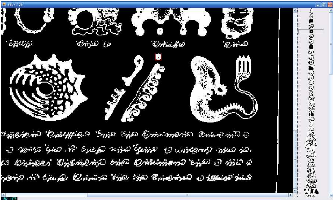
Figure 16: Near the top of the word results are extraction errors. These are not actually words but rather pieces of illustrations. Further research could find a way to filter these out, possibly by black to white ratio.
