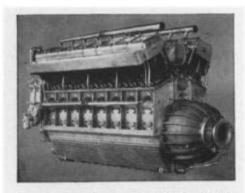
Fig. 6.—Mercedes-Benz DB 602 Diesel airship engine, 1936.
