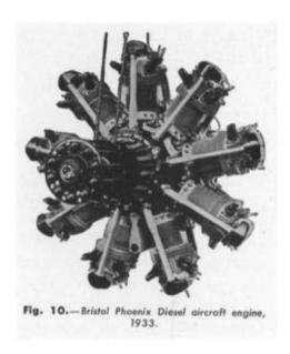
4 per cent (Fig. 11). Its fuel consumption was also reduced by as much as 35 per cent. These improvements were due to the better power output characteristics of the Diesel at altitude (Fig. 12). Recently, further work has been done on the Bristol Phoenix and its crankshaft speed and supercharger impeller speed have been increased so that it is now rated at 635 h.p. at 2,100 r.p.m.
