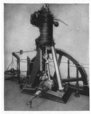
Fig. 2.—First commercially practical Diesel, 1897.
