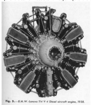
Another Diesel aircraft engine which has been developed in Germany is the B.M.W.-Lanova 114 V-4 Diesel built by B.M.W. Flugmotorenbau. G.m.b.H. (Fig. 5). Dr. Schwager has been responsible for much of the work on this nine-cylinder radial which is moderately supercharged and rated at 650 h.p. at 2,200 r.p.m. This engine, like the radial gasoline engines manufactured by the firm, functions on the four-cycle principle. It is unique in that although it is
