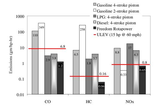
Figure 3: Comparative Emissions Performance<sup>8,9</sup> ULEV is the California Ultra Low Emission Vehicle Standard
