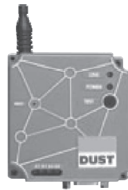
Fig. 30.7.d: Dust Networks Evaluation Mote
