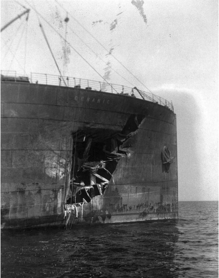
August 1940 At Walvis Bay. Bow end of the Ceramic , showing damage sustained in collision with the Testbank .
