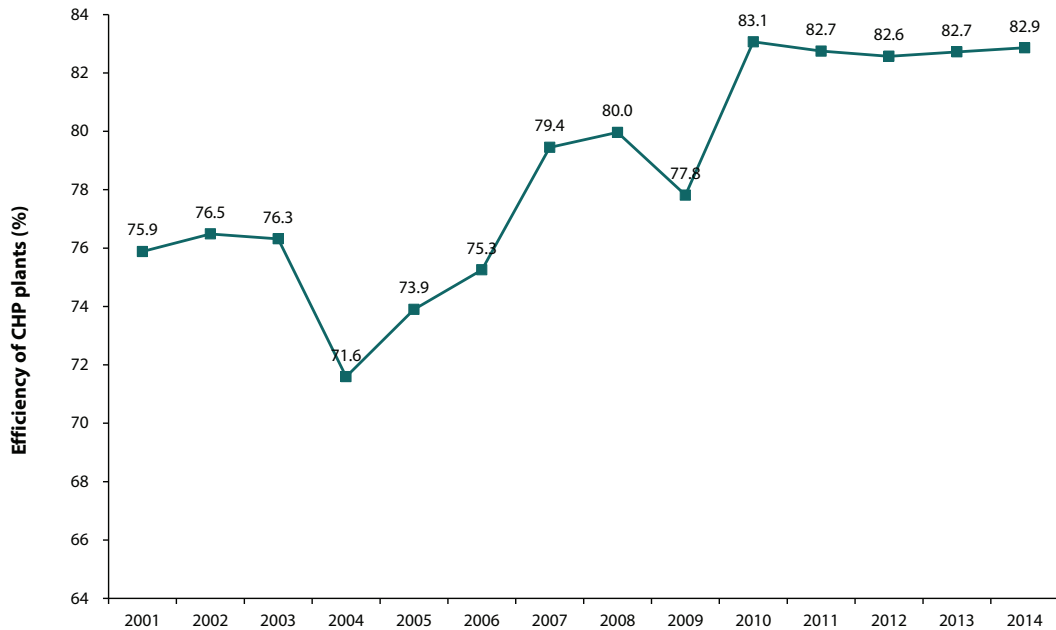
Figure 6 Efficiency of CHP Plants
