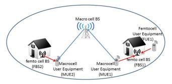
Fig. 2. Inter-cell interference between macro and femtocells
