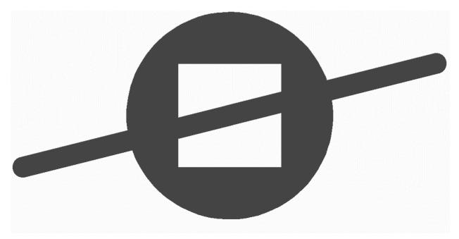
50. Standard (circle) aperture with a rectangular hole above a draw Note that the draw is visible through the hole.
