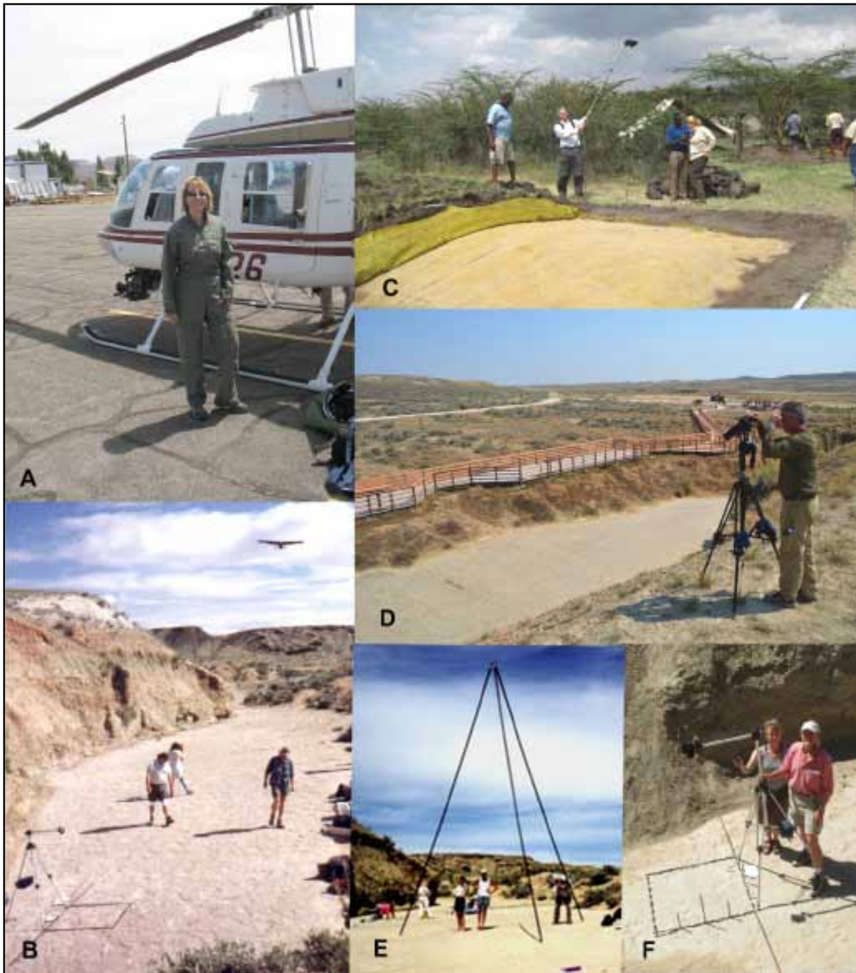
FIGURE 1. A , preparation for low-level imagery collection using digital SLR camera mounted below Bell Ranger helicopter of the Moccasin Mountain Tracksite near Kanab, Utah, summer 2008; B , ultralight image collection over the Red Gulch Dinosaur Tracksite (RGDT), Wyoming, summer 1999; C , monopod mounted camera with remote trigger, Laetoli Hominid Tracksite, Tanzania, spring 2011; D , setting up the Gigapan robotic mount to collect high resolution imagery at RGDT, summer 2012; E , 10-meter tripod used to collect imagery at RGDT, summer 1999; F , 1.5-meter tripod used for imagery collection at RGDT from 1998 to 2001. All BLM photographs.
