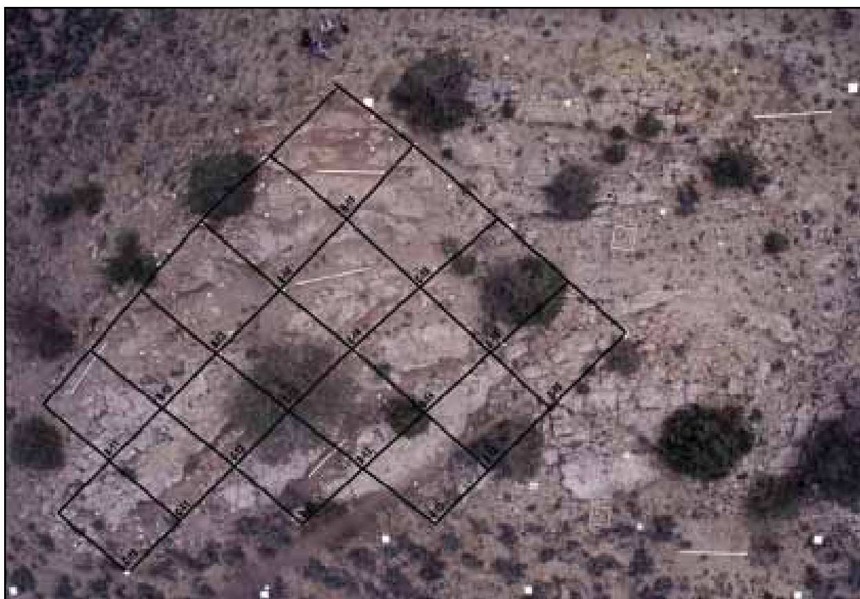
FIGURE 8. Grid created from the aerial photograph using the ACBS. Grids are 5 m (16 ft) squares. Large ornithopod track preserved as a natural cast (Fig. 12) can be seen in the upper right side of the uppermost grid (Grid B15). In addition five standard survey stadia rods and two wooden, two-meter square grids can be seen in this figure. BLM photograph.
