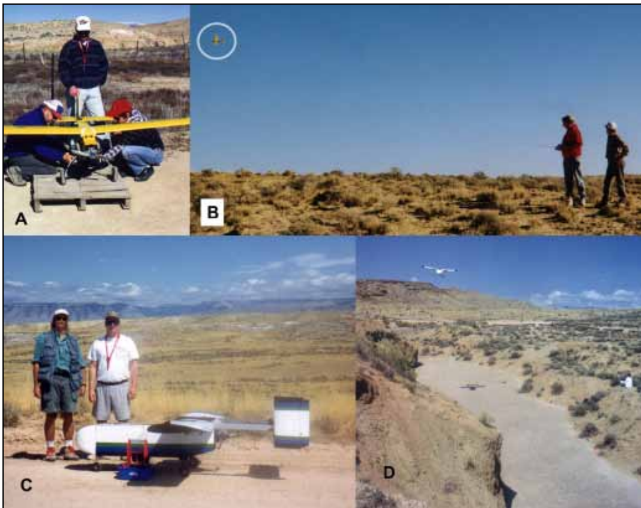
FIGURE 2. Low-altitude, remote controlled airplanes were used to capture imagery at the Red Gulch Dinosaur Tracksite, WY during 1998 and 1999. A , prepping the Senior Telemaster aircraft for flight; B , remote piloting of the Senior Telemaster aircraft (circled in the upper left of image); C , utility styled, aircraft with rear mounted engine; D , utility aircraft flying over them main track surface. All BLM photographs.
