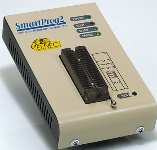
Figure 1. Elnec's SmartProg2 was used for a number of years in the Elektor Labs for one-off microcontroller programming and small series.
