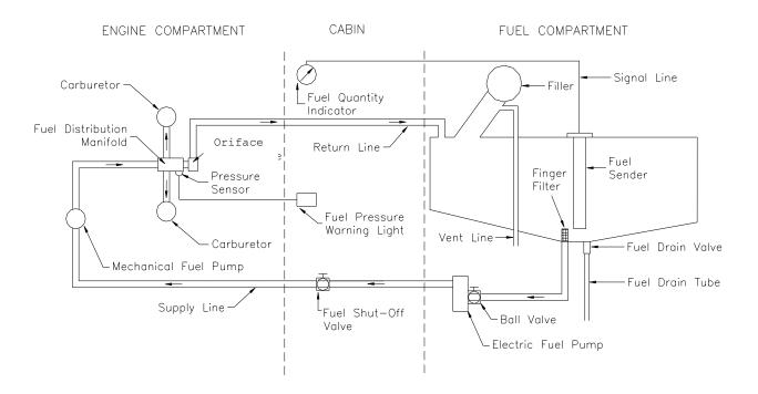
The tank, made from aluminum, is located behind the seats, below the baggage compartment. It holds 76 liters (20.1 US gal.), of which 74 liters (19.5 US gal.) are usable. The tank filler on the left side of the fuselage behind the canopy is connected to the tank with a rubber hose. The tank vent line runs from the filler connection piece through the fuselage bottom skin to the exterior of the airplane.
