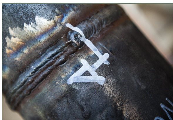
Figure 11: X-ray control of a tank welding (Source: IRSN)
