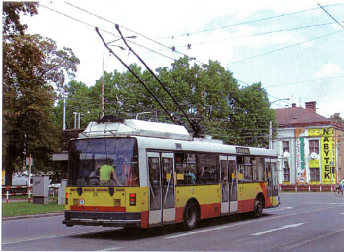
Hradec Králové 50 (a Škoda 21Tr duobus) in service on route 1, which requires dual mode vehicles as there is an unwired extension for some journeys, on 4th September 2006.
