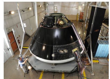
The Multi-Purpose Crew Vehicle being assembled and tested at Lockheed Martin's Vertical Testing Facility in Colorado.
