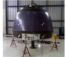
Blue Origin's Composite Crew Pressure Vessel
