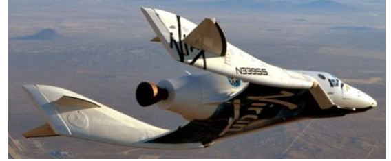
Powered configuration glide test of SpaceShipTwo, December 2012
