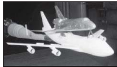
Figure 2. 14-Foot Wind Tunnel model of Space Shuttle Orbiter and 747 aerodynamic test of mated vehicles
