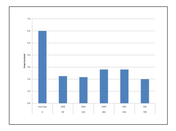
This is the average of the drops survived shown in increasing level of usage Startling all used ropes down to around 2 drops survived on average
