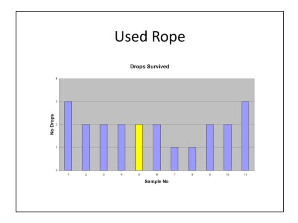
First note variability along length of rope. Shows taking sample from end is unlikely to reflect performance of rope
