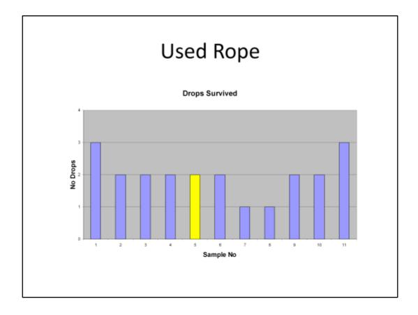
Marks on rope These did not seem to make any difference to the survival rating as the sample with the glaze is number 5.
