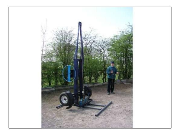
It is a simple mobile rig, some 3.4 metres high and uses a sample of rope around 800 mm long under a load from the test weight of 100 kg.
