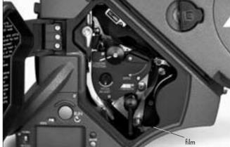
Lock the magazine completely into the camera opening.
