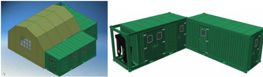
Figure 3. A container workshop project arranged in an L shape
