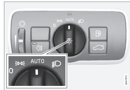
Headlight switch in the AUTO position
