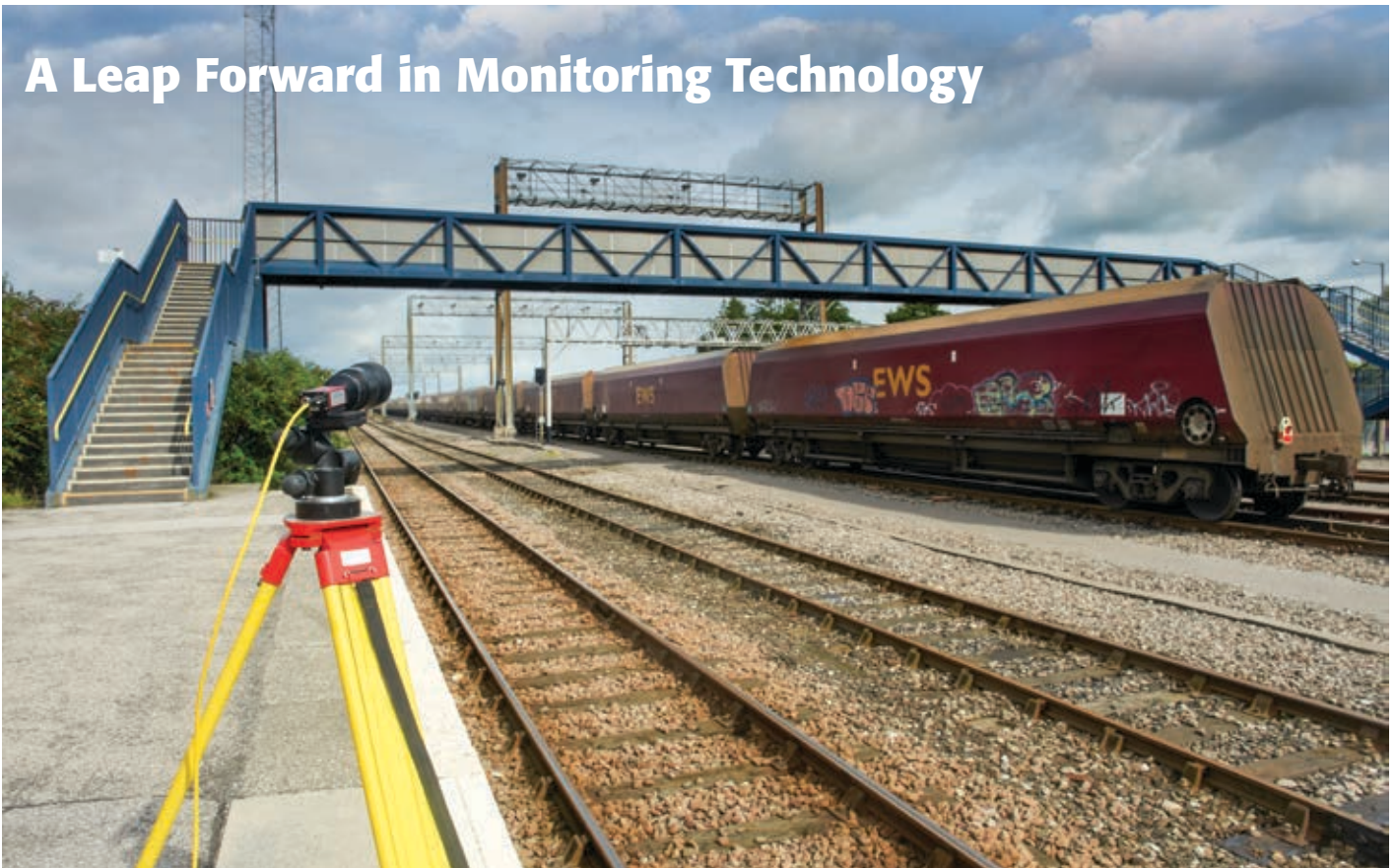
The iMetrum video gauge set up to measure displacement of tracks
