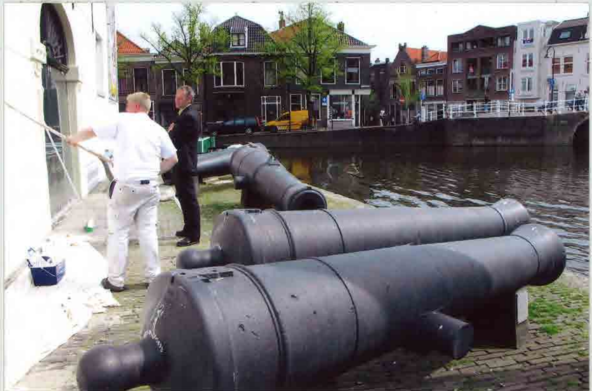
Exhibited outside, these late 18 th century pieces are models originally developed in 1786 for the French Navy. The Dutch adopted them in 1795. Originally, these cannons were shooting massive iron balls of 36 pounds. Around 1830, the piece in the foreground was re-drilled so it could shoot “granaten” or explosive shells of 20 cm diameter. It is marked n°35 (its serial number in the Navy) and, on the breech mouldings : “36 Lb” and “1809” (the year it was cast).
