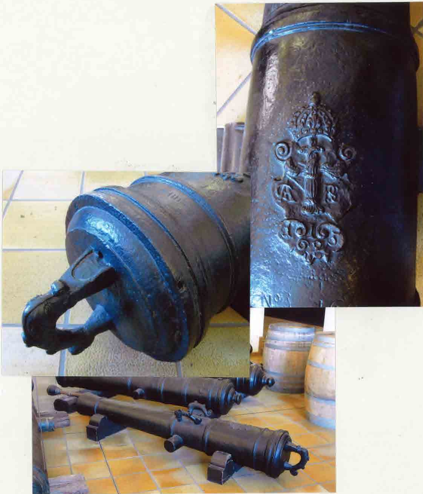
This 17 th c., Swedish gun is not what it seems to be. It is actually a breech-loader. The breech and the whole cascable part, from the base ring on, is mobile and can be unscrewed for loading purposes. This was probably achieved with the help of a cross-lever applied to the delphinoid tail-ring or with tools applied to specially made (square) holes (provided in the base ring). The gun bears the arms of King Gustavus Adolphus of Sweden (1594-1632), the date of casting: "1625" and a serial number : "N° 169". The touch-hole is pierced through the base of the breech moulding (which is unusual) and its powder pan is cut in the upper part of the tail-ring.
