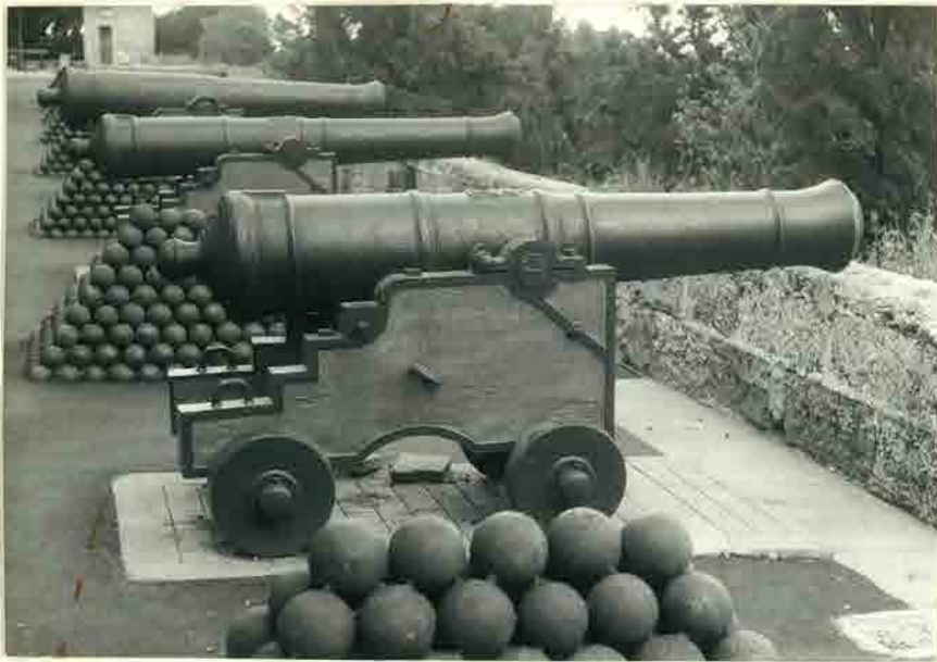
Monaco # 5 British iron ship or fortress gun Cypher of George 2 Caliber 4 1/2" length 98" 1727-60
