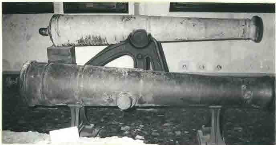
Venice #23 (#3646) French iron naval gun Dated "An 12" cast at Creusot works Caliber 14 Cm Length 285 Cm
