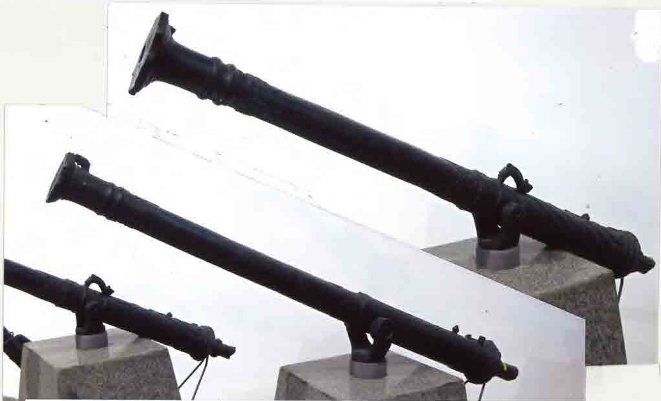
Two “Falconetti de Murata” or “Bulwark falconets”. These bronze small calibre muzzle loaders were actually used on ships, as well as fortifications. The cabled breech, the floral decoration and the typical wide and flattened mouth seem to ally these pieces with the Lanteka family. The notice plausibly indicates that “they probably come from Goa”
