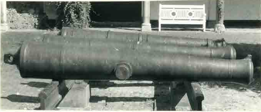
Leiden # 46 Dutch iron gun Caliber 16.5 Cm Length 288.5 Cm Signed on right trunnion: "LUIK 18-3"
