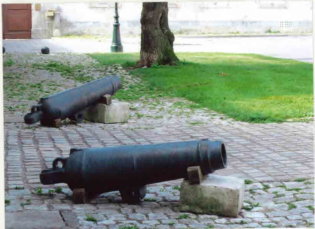
Two cast iron French made, early 19 th century carronades (in front of the museum) and inside, a fine model of a similar "carronade de 30". (The model is at scale 1/6). The model shows a 30-pounder, 1.70m. long, weighing about a tonne. A muzzle-loader, which the arrangement shown on the model obliged the gunner to clean, to cool and to recharge the piece from the outside of the hull, precariously standing on a special narrow support.
