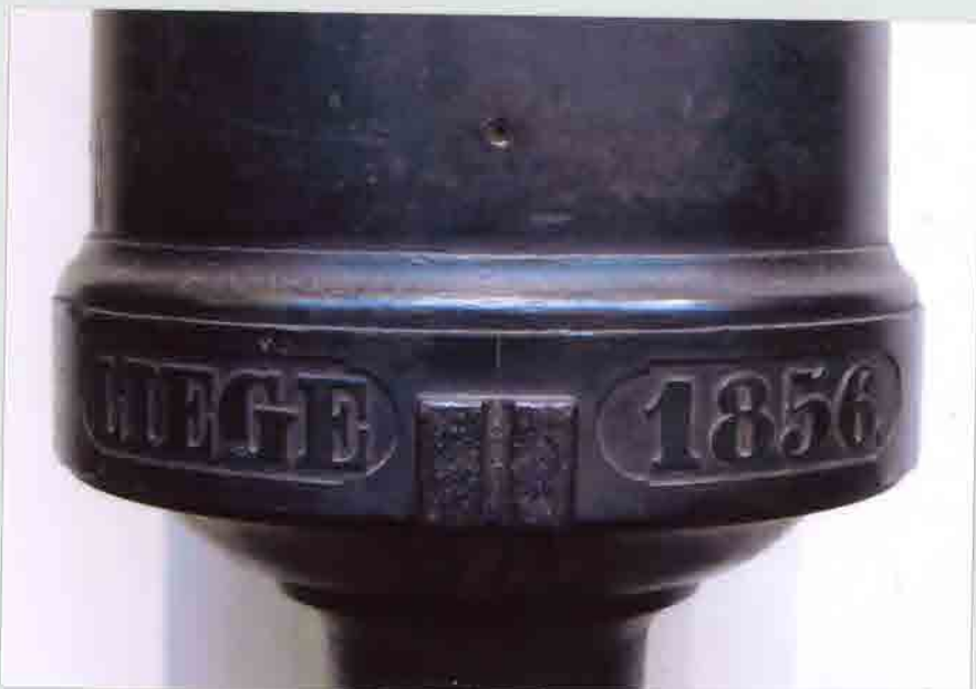
Bronze short gun cast in Liège in 1856, as indicated on the base ring (with a moulded sight between the place name and date). The cascabel is a simple, solid cylinder.
