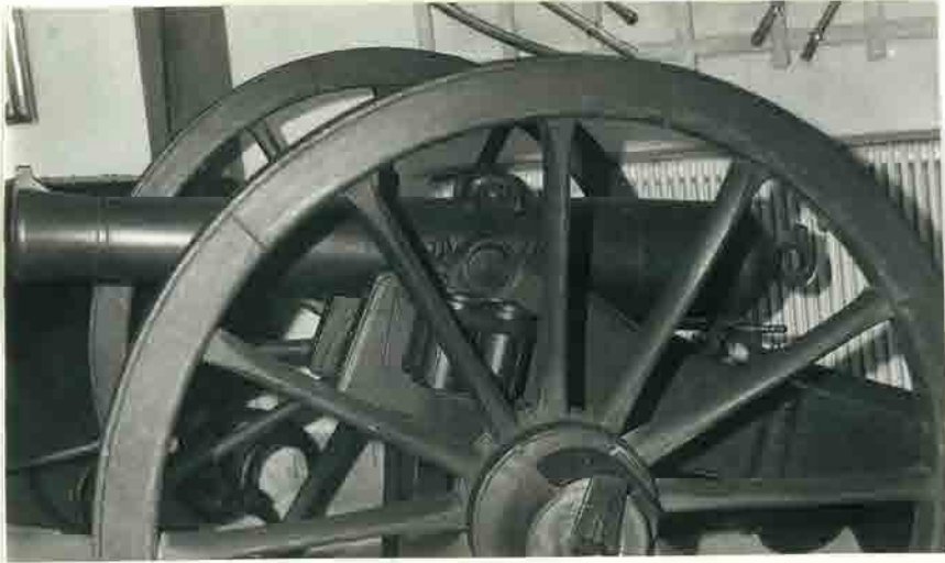
Leiden # 35 Dutch bronze fieldpiece Caliber 8.5 Cm Length 162.5 Cm Signed "MARITZ ET FILS PRO HAGAE A o 1843"
