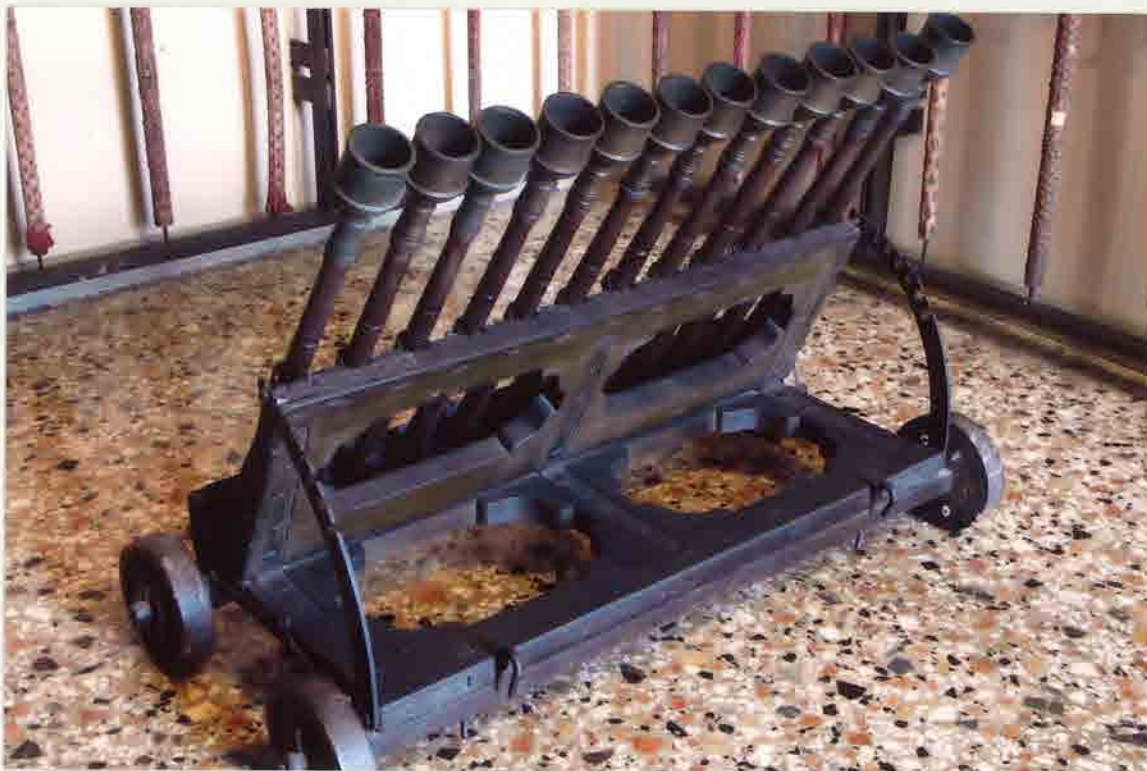
A "macchina" (a machine or device) with twelve firing mouths, called "organo" (organ) of the XVII century – Probably an experimental piece, meant for siege operations and to be used to fire grenades or incendiary bombs (?) over walls. It consists in fact, of a row of 12 miniature mortars, fitted on as many stocks.
