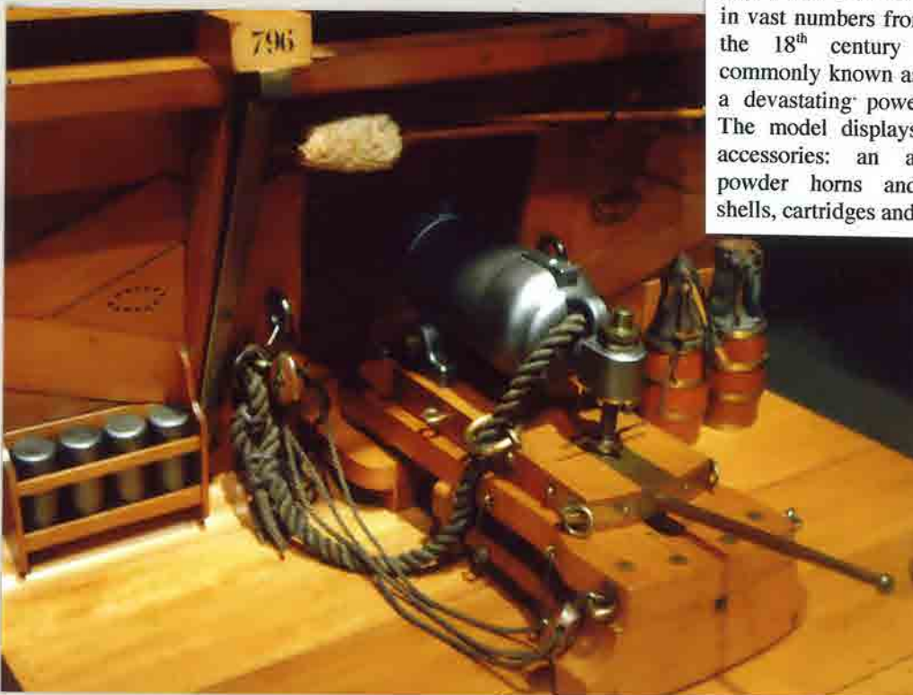
A ship's mortar on its rotating support in the hold of a "mortar ship" or "bomb ketch" or "galiote à bombes". Such weapons were used from a well anchored ship against land fortifications or against an enemy fleet at anchor and enjoying the protection of a closed harbor.
