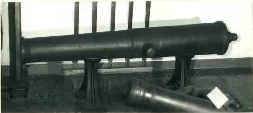
Venice #12 (#141) Bronze "Aspide" 12 pounder, used at Famagosta in 1571. Cast by "GALFACIUS ALBERTGHETTI" Caliber 10 Cm Length 185.5 Cm
