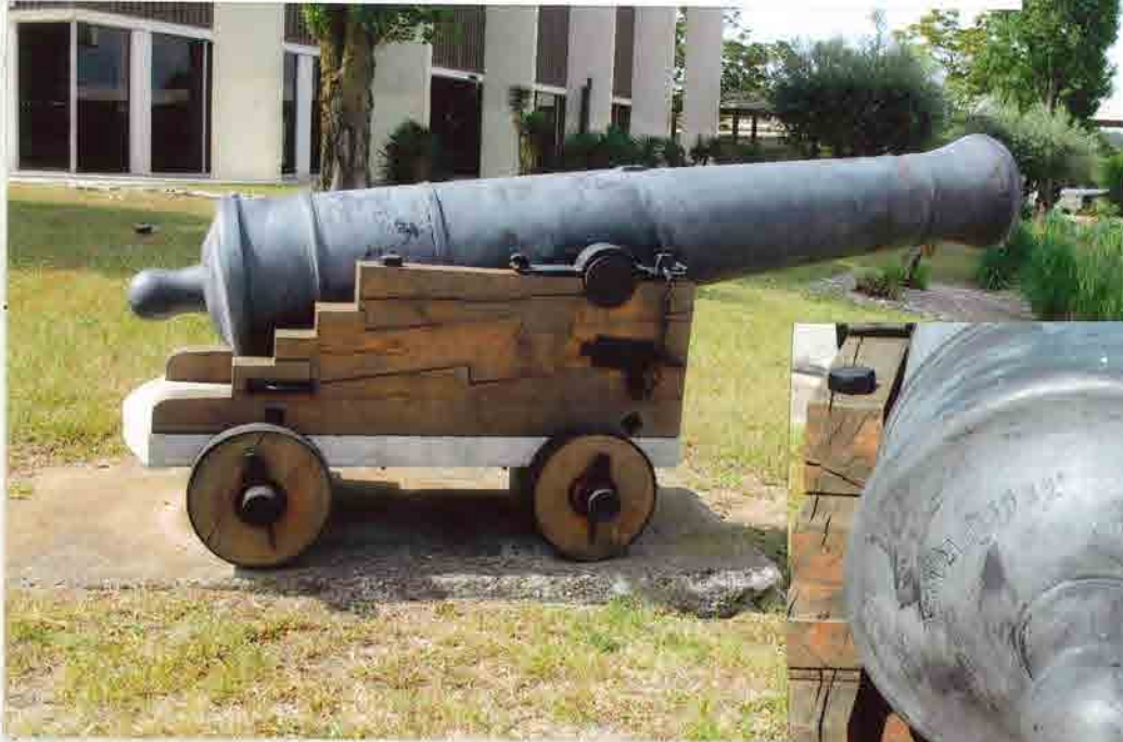
Cast iron naval piece. Calibre: 16cm; weight: 3,089 kilos. Cast in 1811 in Sant-Gervais, France.
