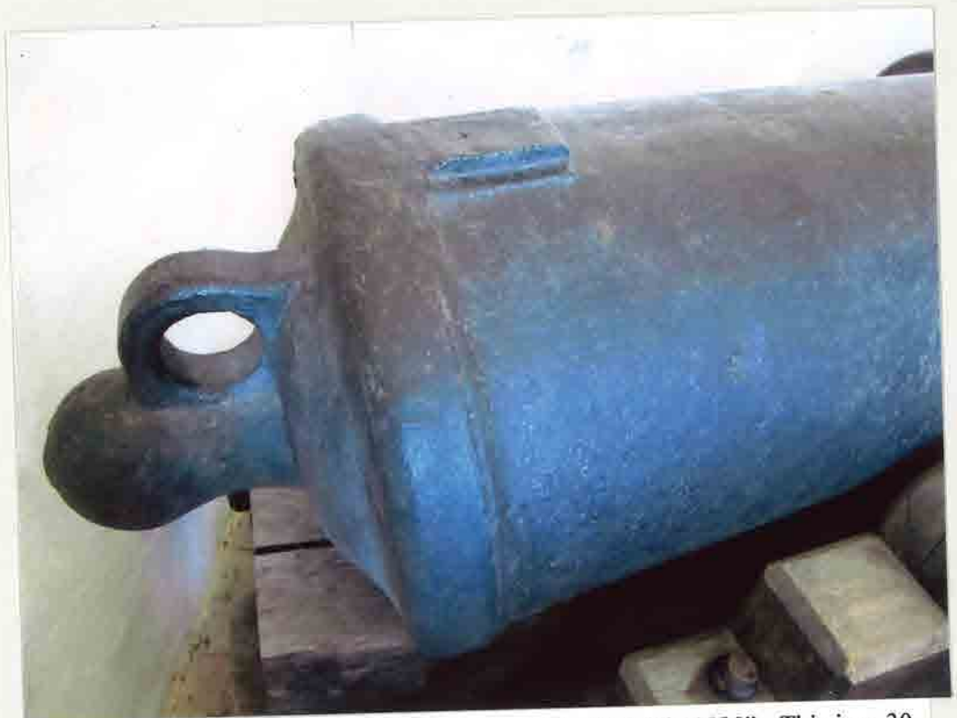
"Canon de 30 court", the short 30-pounder of the "Modèle 1820". This iron 30-pounder is a new calibre, introduced by still another reformer or systems inventor, the Lieutenant General Thirion, Inspector General of the Naval Artillery. The 1820 new rules introduce the English innovation of the annular top of the breech button (to accommodate the anti-recoil cable).
