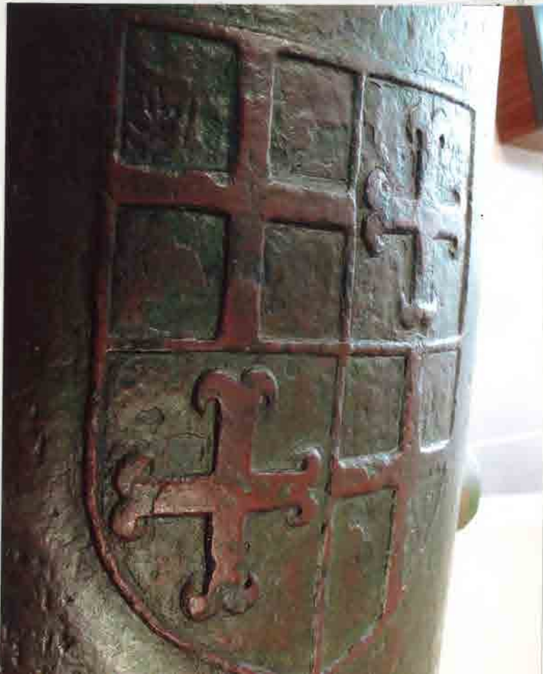
Dimensions: Calibre: 58cm., length: 1.95m.; (piece called "for 500 pounds of stone ball"); weight 3,325 kilos.
