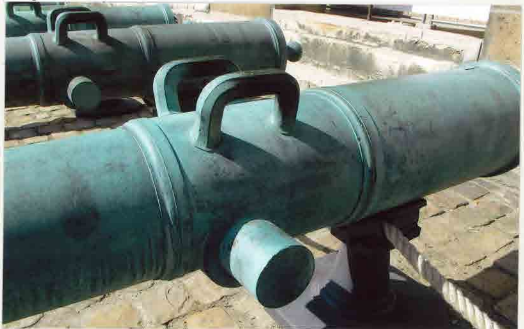
"L'AMÉ" (The Well Loved). 24-pounder cannon of the Gribeauval System, "modèle 1775". Cast in Strasbourg in 1832 and was rifled sometime in the 19 th century. Weight: 2,750 kilos.
