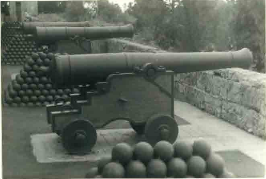
Monaco # 7 French iron gun Caliber 4\frac{1}{2} " Length 109" "I.R." on 2nd. reinforce Star and "No 1254" on base ring
