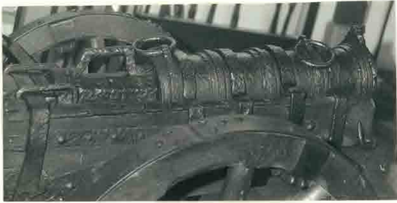
Leiden // 11 Wrought iron field piece on carriage Caliber 17.5 Cm Length 111 Cm Late 15th. century
