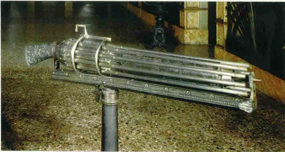
Early prototype (exact date uncertain) of a machine gun-like weapon. It has 10 barrels, each with its individual chamber for cartridge and projectile.
