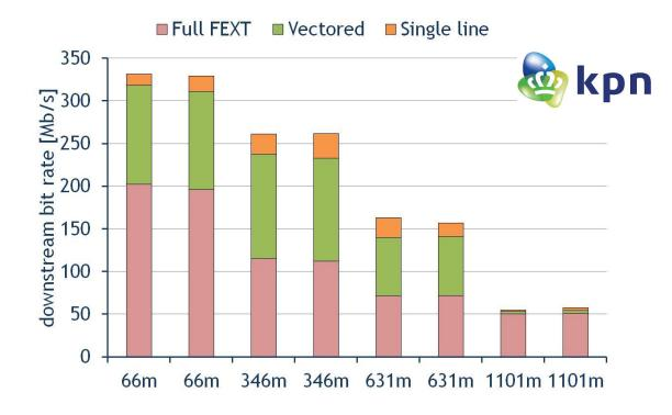
Record copper in test environment with new technology
