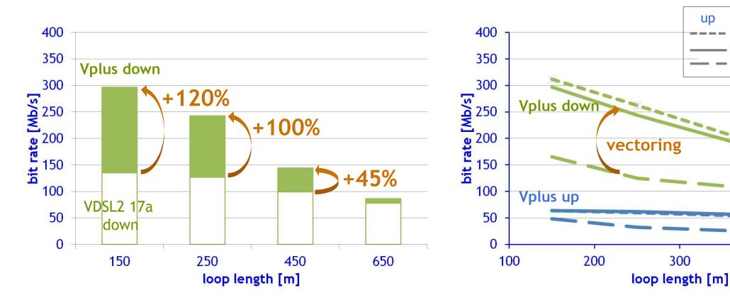
Operator cable; mix of VDSL2 17a and Vplus (35b) in same cable with distributed loop lengths
