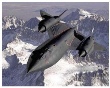
SR-71 flying across the snow-covered southern Sierra Nevada Mountains of California after being refueled by an Air Force tanker during a 1994 flight. This picture shows the corrugation on the wings and the angle of the vertical fins.
