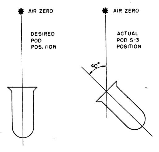
Figure 2 - Pod Position Diagram
