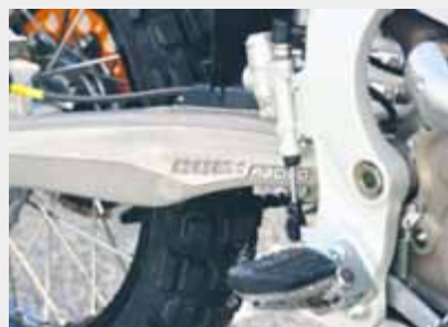
Engine mounts are blamed for excessive vibrations. CCM will be replacing them
