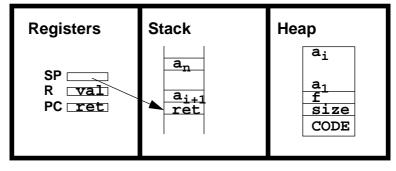
What the cleanup code did was to bring the stack back to its original state and to delete the return structure. The **D0** register contains the return value from function  $\mathbf{f}$ , and the program counter will branch back to the original caller.
