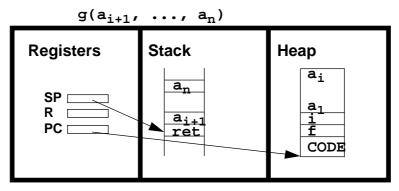
The curried function  $\mathbf{g}$  is called with some parameters. The above picture shows the situation just before branching to  $\mathbf{g}$ . As for any normal function call, the parameters have been pushed on the stack. The program counter points to the structure on the heap, so the next instruction to be executed will be CODE.
