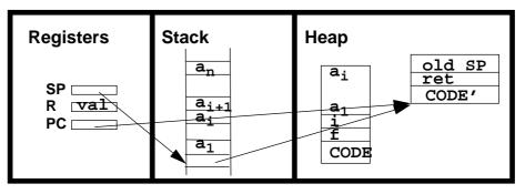
The function  $\mathbf{f}$  is going to return, so the program counter contains the return address that was on the stack. As we saw before, this is the address of some cleanup code in a return structure. The  $\mathbf{R}$  register contains the return value from function  $\mathbf{f}$ .
