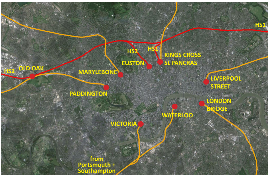
fig. 13. The London terminals, showing programmed HS lines (red) with other primary routes out of London Rail
