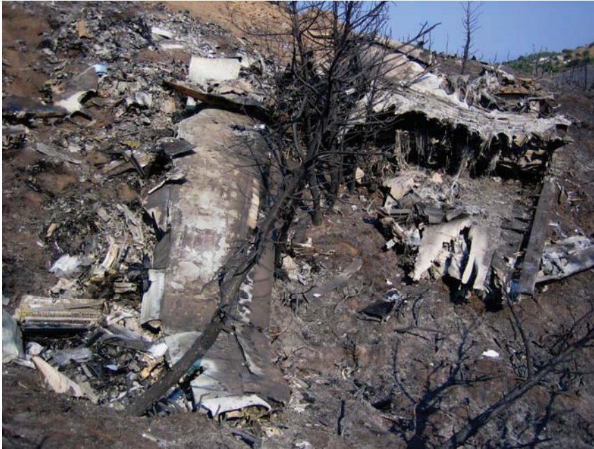
Photo – The right wing tip is at the lower left and the left wing is at the right edge of the photo. The center section and main gear well is at top right.
