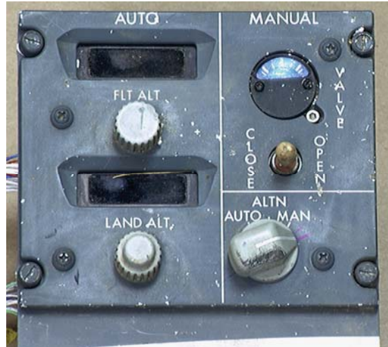
Photo – Pressurization Panel
