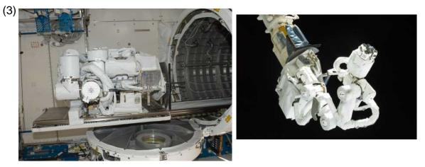
Figure A2-10 Small Fine Arm (SFA) of the Kibo's Remote Manipulator System (JEMRMS) (Delivered by the HTV1)
