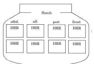
Figure 4.1-1 Rack layout in the HTV4 PLC
