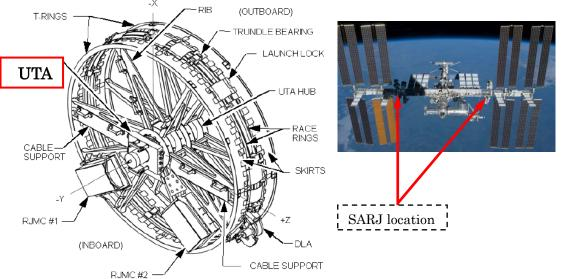
Figure 4.2.1-6 SARJ structure (From NASA STS-115 Press kit)
