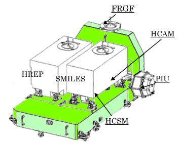
Figure A1.3-2 Exposed Pallet for EF Payload (Type I) (Note: Configuration for the HTV1 Mission)
