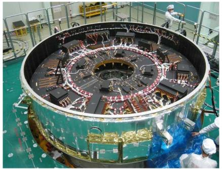
FigureA1.4-2 Avionics Module (Top View) (HTV2)
