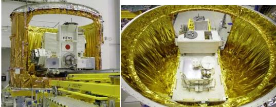
Figure A1.2-2 EP Being Loaded Figure A1.2-3 EP Installed into the ULC (HTV3) (HTV3)
