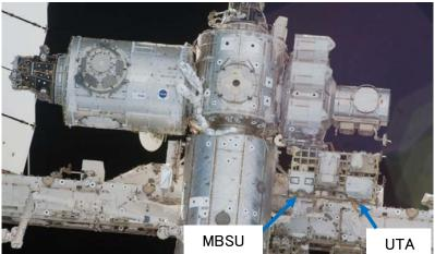
Figure 4.2.1-5 MBSU and UTA spare parts (covered in thermal insulating covers) stored on the ISS ESP-2 (Photo courtesy of NASA. Photo taken after STS-130 mission)
