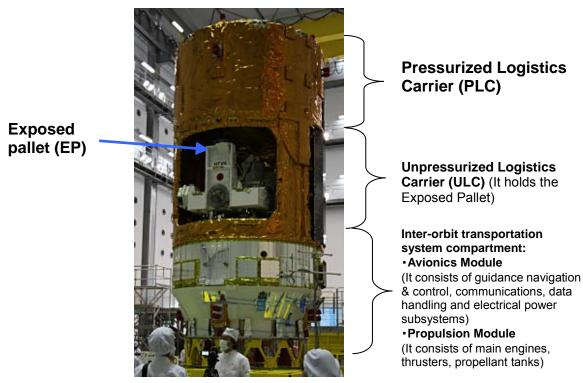
Figure 1.1-1 Configuration of "KOUNOTORI" (photo: HTV4)
