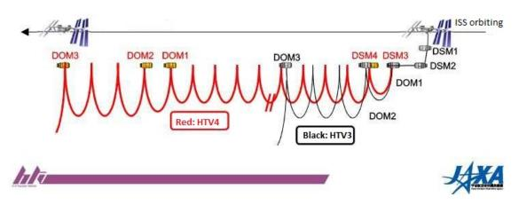
Figure 5.1-2 Trajectory differences with the HTV3 and HTV4 In the HTV4 mission, in order to shoot the reentry of the HTV4, Descending Maneuver (DSM) 3 and 4 will be added to let the HTV4 descend and fly single Earth orbit ahead of the ISS. At the timing of the HTV returns and flies below the ISS, HTV's De-Orbit Maneuver (DOM) will be performed.
