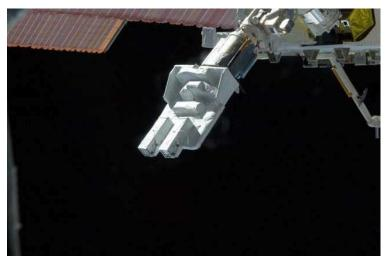
Figure A3-6 Grappled by the Kibo's RMS, the J-SSOD is ready to release CubeSats
