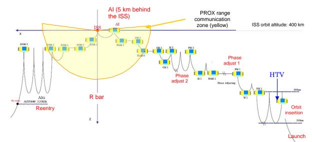
From 90 minutes before the HTV reaches the AI point, HTV integration operations by the HTV MCR and the Mission Control Center at NASA's Johnson Space Center (JSC) in Houston (MCC-H) will begin. The HTV may have to adjust and reschedule its flight timeline up to 24 hours during the rendezvous phase since the HTV proximity operation will have to be performed during ISS crew on-duty hours.
