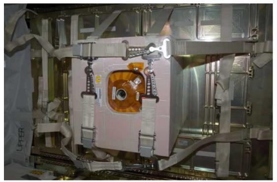
Figure A3-1 i-Ball installed on the PLC of the HTV3 (Before closing the hatch, astronauts strap it and turn on the power)
