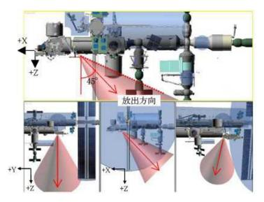
Figure A3-7 Images of CubeSats release operations and release angles
