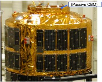
Figure A1.1-1 PLC exterior (HTV1)
