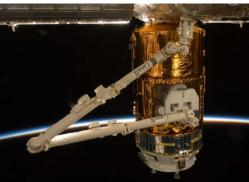
The SSRMS removing the EP from the ULC
