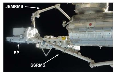
The EP being handed over from the SSRMS to the JEM Remote Manipulator System (JEMRMS) for temporary installation on the EF (image of HTV1)
