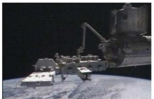
EP being temporally installed to the edge of the EF (HTV1)
