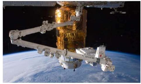
EP being reinstalled into the ULC (HTV3)
