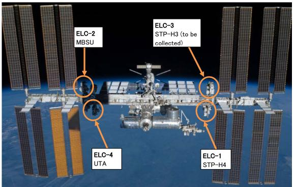
Figure 4.2.3-3 Installation location for each equipment to be delivered and collected by the HTV4 mission (courtesy of NASA)
