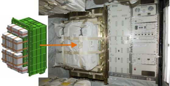
Figure 4.1-4 Left: CTBs installed at the front of a rack (HTV2) (Right: KOBAIRO Rack)
