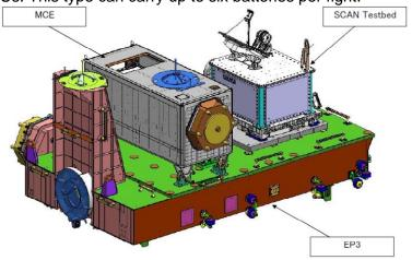
Figure A1.3-3 Exposed Pallet-Multi-Purpose (Type EP-MP) (HTV3 configuration)
