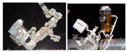
Figure A2-8 US ORUs: (Flex Hose Rotary Coupler: FHRC) and Cargo Transport Container: CTC (Delivered by the HTV2)
