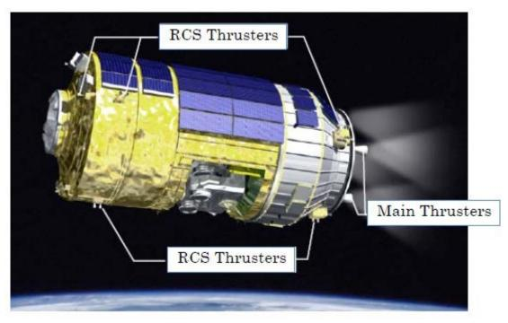
Figure A1.5-4 Locations of Main Engines and RCS Thrusters
