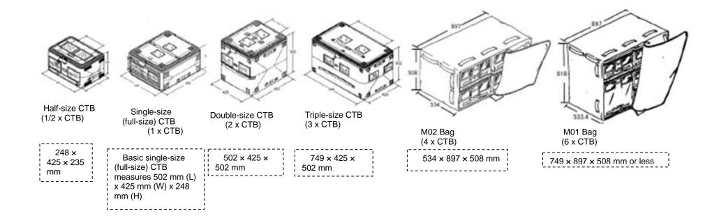
Figure A2-1 Several sizes of CTBs are available to transfer goods to the ISS
