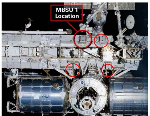
Figure 4.2.1-1 Four MBSU installed on the S0 truss of the ISS (Photo: NASA)
