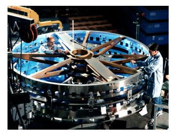
Figure 4.2.1-7 SARJ rotating ring (Photo courtesy of Lockheed Martin)
