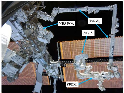
Figure 4.2.3-1 A US payload being transferred using the SPDM (FHRC transfer on the HTV2 mission) (Photo courtesy of NASA)
