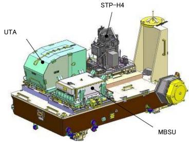
Figure 4.2-2 Cargo loaded on the EP (HTV4)
