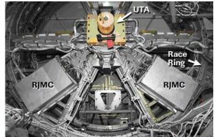
Figure 4.2.1-4 UST installed to the center of SARJ (Photo courtesy of NASA)
