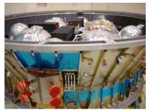
Figure A1.5-1 Propulsion Module (Before installation of MLI covers)
