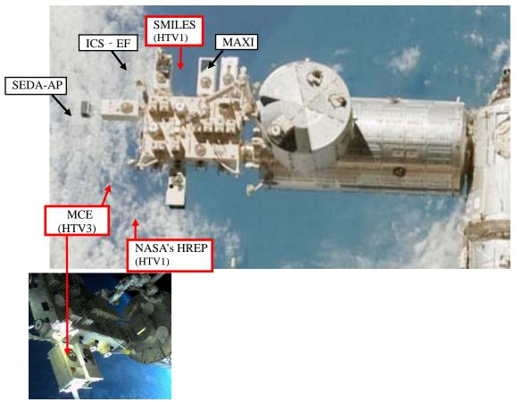
Figure A2-7 EF payloads delivered by the HTV1-3
