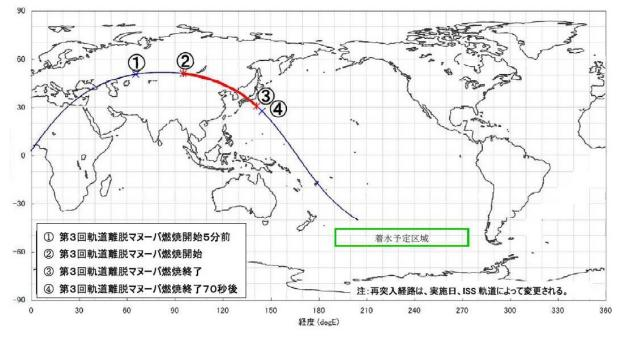
Figure A2-4 HTV's projected reentry path Expected deorbit burn duration (red line) and HTV splashdown area (green box)
