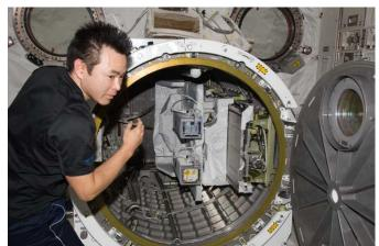
Figure A3-5 MPEP and J-SSOD installed in the Kibo's airlock
