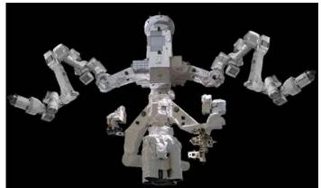
Figure 4.2.3-2 SPDM called "Dextre" (Credit: NASA/CSA)
