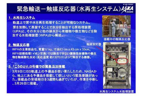
Figure A2-15 Catalytic Reactor (a part of Water Recovery System (WRS)) delivered as expedite shipment upon a request from US (Delivered by the HTV3)
