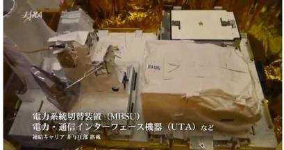
Figure 4.2-3 UTA and MBSU loaded on the EP (HTV4)
