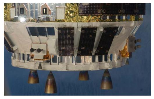
Figure A1.5-3 Propulsion Module Photographed from the ISS (HTV1) (Four nozzles seen in the bottom are main engines)
