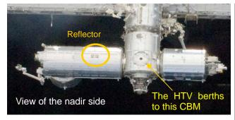
The Laser Rader Reflectors (LRRs) are located on the nadir side of the PM. The reflectors will reflect the lasers beamed from the HTV's Rendezvous Sensor (RVS) when the HTV approaches from the nadir side of the ISS.
