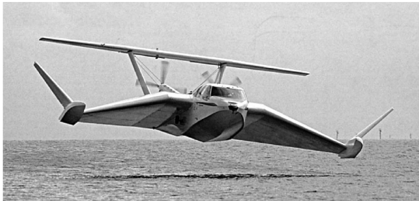
Fig. 1. A WIG craft recently introduced to operation by Pacific Seaflyght on Alaska
