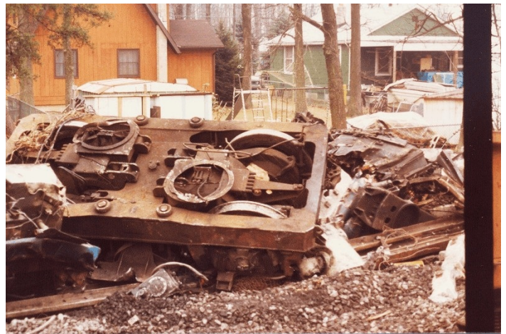
GUNPOW: A WEEK AFTER THE COLLISION. A TRUCK FROM ONE OF THE DESTROYED AMTRAK AEM-7S PUSHED TO THE SIDE OF THE RIGHT-OF-WAY. PHOTO BY GEORGE PITZ, AMTRAK - USED WITH PERMISSION.
