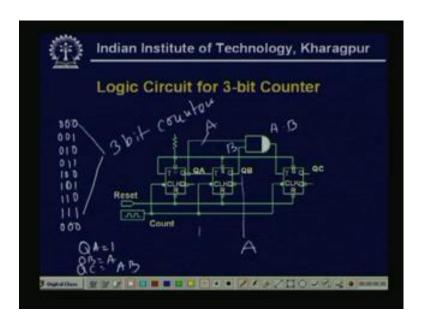
If we see the design, then see, that first we have taken 3 D flip-flops, here we have constructed the logic circuit by D flip-flop. Then see, as usual the reset lines and the clock lines are there, then Q A value, here the Q A value is always 1. So, this is my, this is my T A value or the first one. See the Q A is A means the previous input and Q C, see this is my, this is my A and this is my B, so this is my A dot B and that is my Q C.
