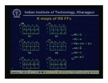
So, depending on that, now we will get the, as for the three flip flops and now there are two outputs R and S. So, for the C flip-flops, what will be the R C S C, for the C B flip flop, what will be the R B S B and for A, what will be the R A S A. So, the based on the, the remapped next state, that Karnaugh maps have been filled up. Now, if that, we do that Karnaugh map minimization, we will be getting that this type of logics. We will be
