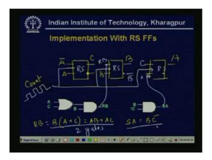
So, now if we start drawing, so first we need three R S flip flops, so this is one, actually this is my C this is Q bar, so this should be A bar, this should be my A, this is the B, B bar, C and this is A and C. The clock line is these are the, so this is the clock or we can tell, this is my, this is my count. Because, at each clock it will generate one state; that means, it will 1 one count will be going on. So, this is my, this output is my R B, this is my B bar and this is my A B C.
