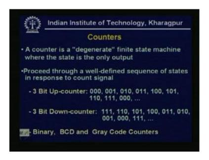
Now, if you see the counters, now a counter we can define in this way the counter is a degenerate finite state machine, where the state is the only output. So, there is no other
