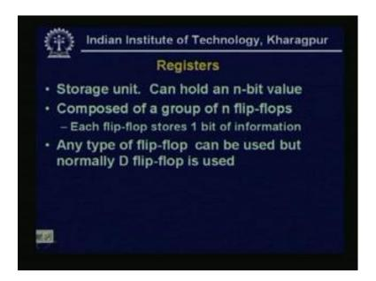
So, this is a storage unit and can hold an n bit value, so first we will see that how or 1 bit memory element means, 1 bit flip flop. So, how that n bit storage element can be constructed from this 1 bit memory element. So, this is nothing, but it can be composed of a group of n flip flops and each flip-flops stores 1 bit of information. So, this together it will store an n bit information.
