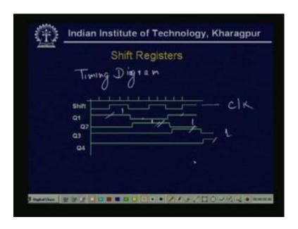
Then, the timing diagram of, see this is the shift clock, so this is my clock, then the four outputs Q 1, Q 2, Q 3. See that Q 1... this is at the high to low because, Q 1 becomes 1 and this becomes 0 when it is a. That means, again when it is a high to low it will be getting 1. Now, again Q 2, Q 2 will be taking, Q 2 is that just the reverse of the Q 1.
