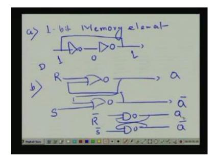
We have read in the last lecture that, the 1 bit memory element, that is by using inverter 1 NAND gate and if it is cascaded with another inverter; that means, 1 NOT gate and another NOT gate. So, if 1 is given as the input, then this 0 is there and then again by using this 1 that means, if this is my data, again this becomes my data and this is feedback as the. So, this is the sample, by using the NOT gate, NAND using the NOR gate we have seen, that two cascaded NOR.
