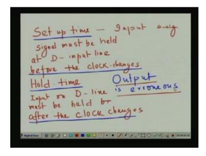
So, first if we think the setup time, the input signal must be held at D input line before the clock changes, so this is my setup time. So, mainly here, before the clock changes and if it is hold time, then already we have seen that it is the same thing. That input on D line must be held before the, this is before the, if it is before the clock changes, then it is setup time, if it is after the clock changes, then it is hold time after the clock changes. So this is after the clock changes.
