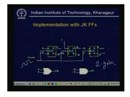
See here K B is A C K B is A C and J A is B C bar, so that means, if we again this is my clock. So, this is my clock and it is shared to three flip flops then this is my A and this is A bar this is my A this is A bar J A C B this is 1 C A, A bar C bar. So, in this case we need 2 extra gates 2 extra gates with JK flip flop, now if we do the implementation with D flip flops.
