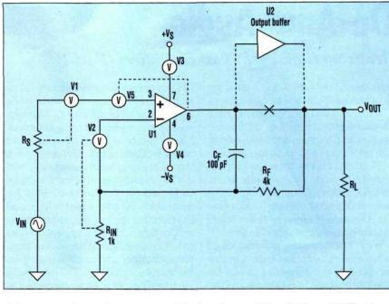
sitic suppression resistances, etc.; this will be an individual thing. There should almost always be some sort of isolation impedance between the buffer output and the output terminal, to isolate any cable capacitance. This can either be a small, 20- to  $100-\Omega$  resistor, or the LR network described in Reference 4.
