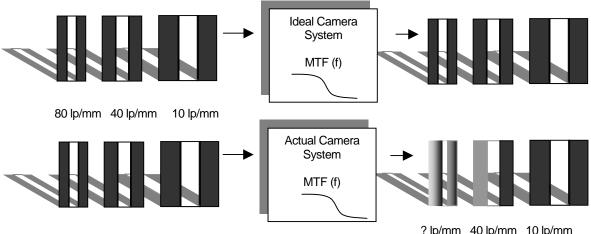
Figure 12 Modulation Transfer Function
