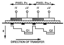
Figure 9 True 2-Phase CCD Cross Section
