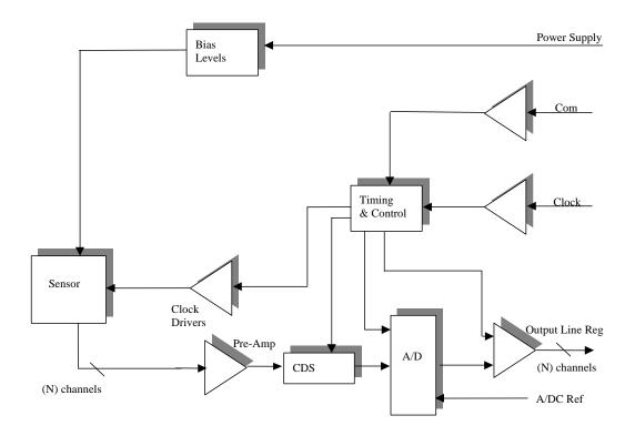
Figure 3 CCD Camera Building Blocks
