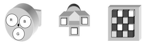
Figure 17 Methods for Generating Color with CCDs
