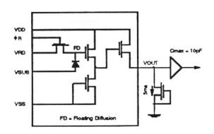
Figure 10 CCD Output Structure
