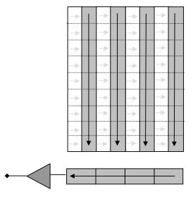
Figure 6 Interline Sensor Architecture
