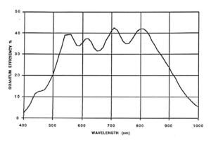
Figure 18 Typical CCD QE Curve
