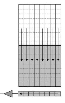
Figure 5 Frame Transfer Sensor Architecture
