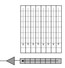
Figure 4 Full-Frame Sensor Architecture
