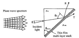
Fig. 1. Thin-film filter for spatial frequencies assembled with a multilayer stack upon a glass prism;  $\theta_{\rm prism}$  is the angle of the prism,  $n_M$  is the index of refraction of the incident medium, and  $n_{\rm sub}$  is the index of the substrate medium.
