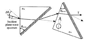
Fig. 3. Bandpass spatial filter assembled with two edge thin-film spatial filters like the filter shown in Fig. 1. The second prism is rotated by  $\phi$  to control bandwidth  $\Delta \theta$ .
