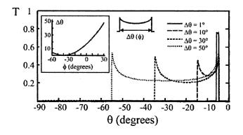
Fig. 4. Transmittance of the bandpass filter shown in Fig. 3. The design of the edge filters is that which was analyzed for s polarization in Fig. 2. Bandwidth  $\Delta \theta$  is variable with angle of prism rotation  $\phi$ .
