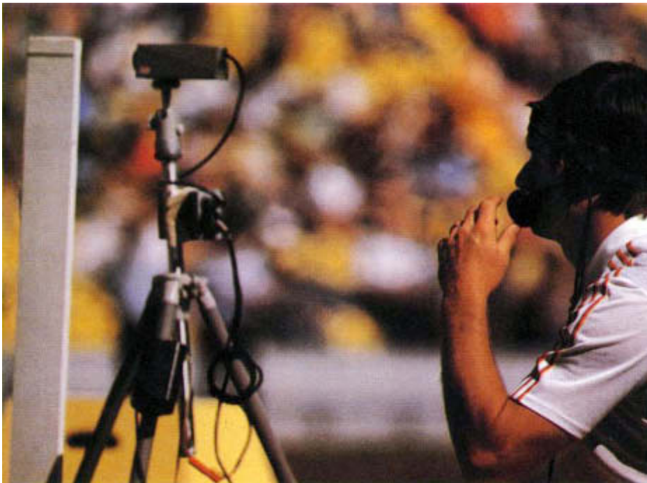
The photoelectric cell which automatically stops the clock on a board and activates a printer when a competitor finishes his event.
