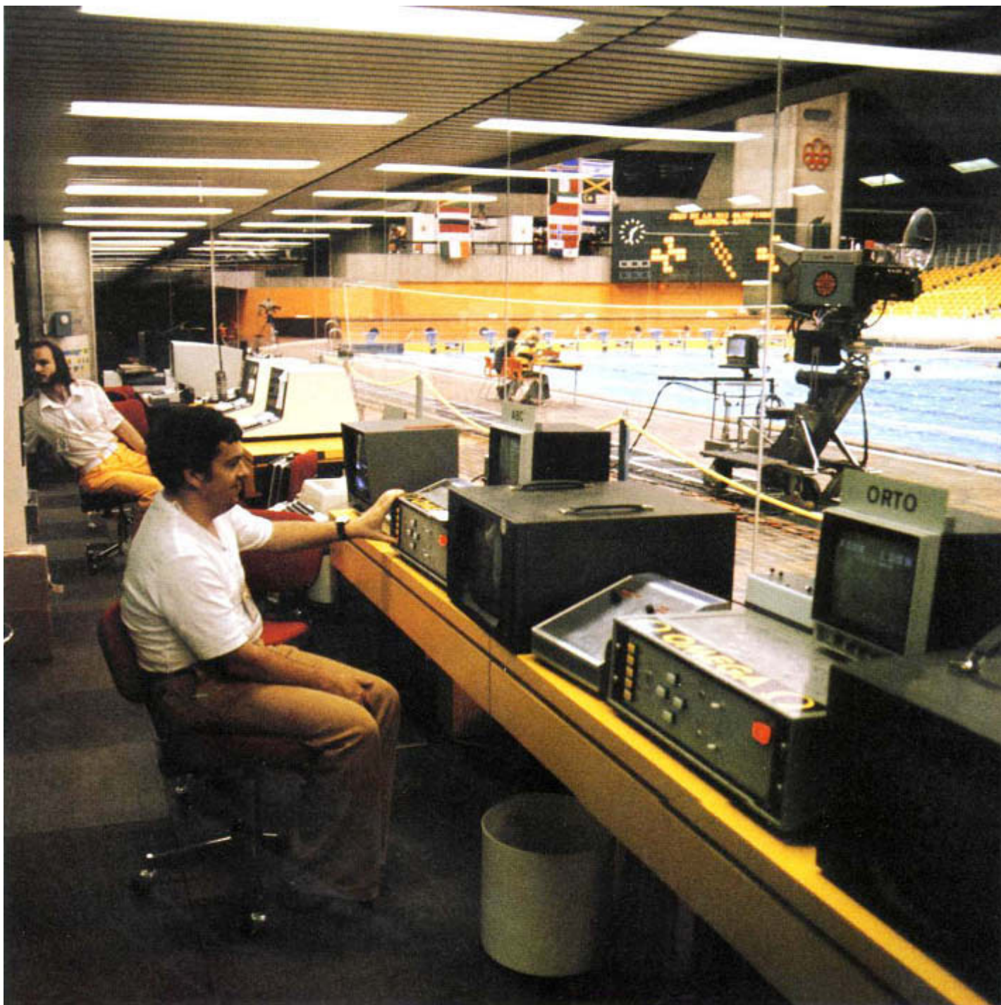
Technology in action: in the main control room at the Olympic Pool showing the equipment used for time-keeping, scoreboard control, and results input.
